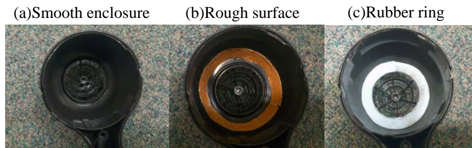
Figure 2.6: Different back enclosure at the inlet:(a) Original smooth enclosure (b) Rough surface at the inlet (c) Enclosure with rubber ring at the inlet
