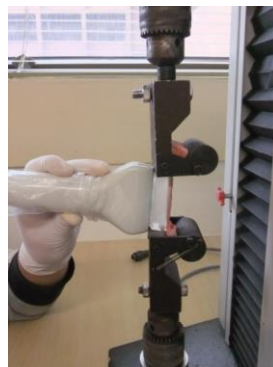
Figure 2.2 Experiment set-up. The gel pad and transducer were put lightly on the tendon in order to capture its elasticity using Supersonic Shear Imaging.
