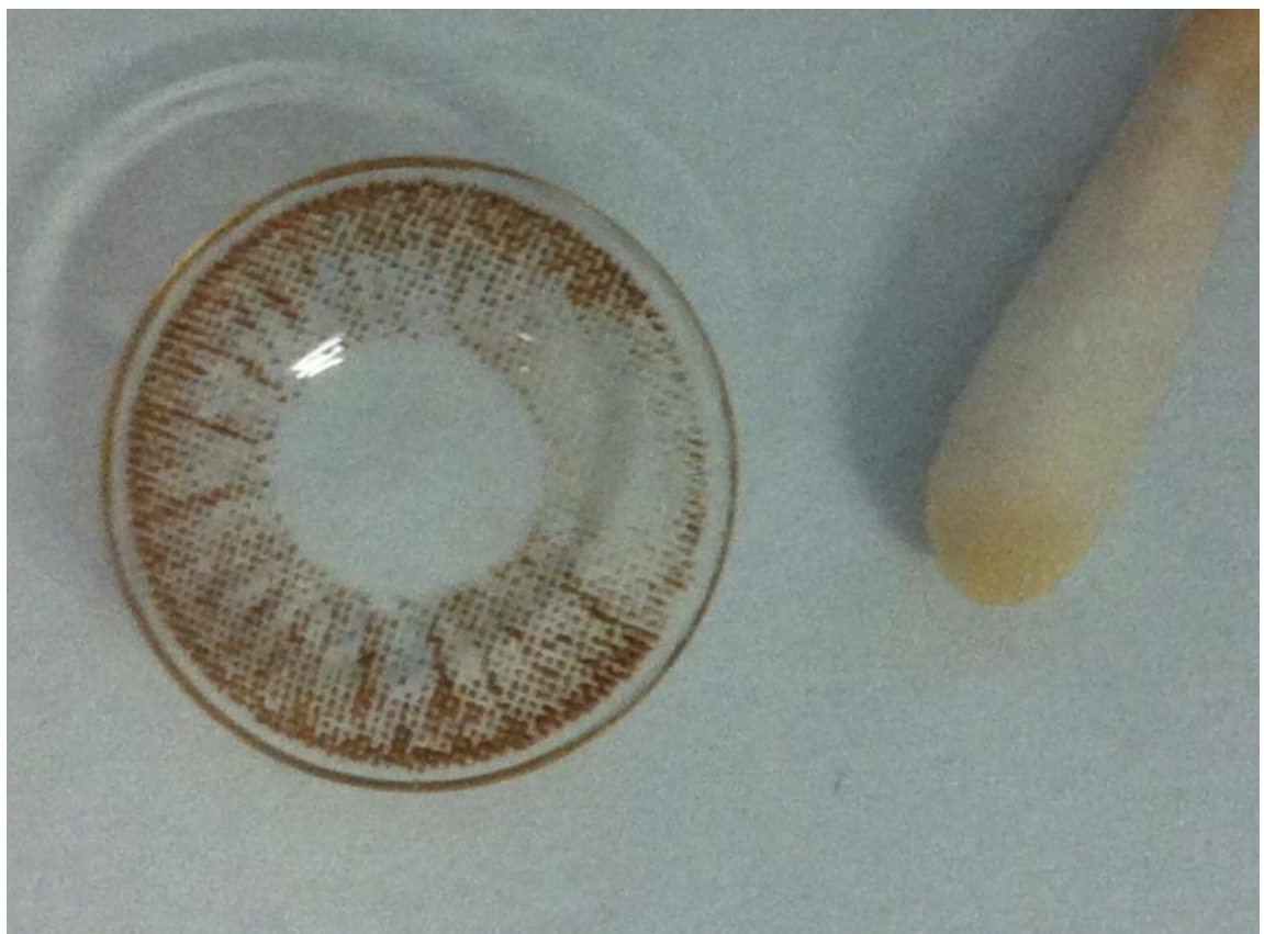
Figure 3.2 Pigments of a cosmetic contact lens transferred to a cotton bud during the rub-off test
