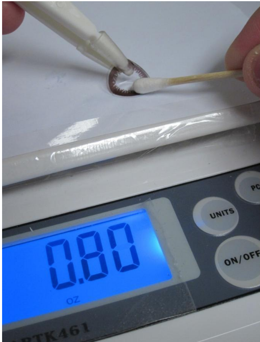
Figure 3.1 Rubbing the front surface of a cosmetic contact lens with a wetted cotton bud on an electronic balance
