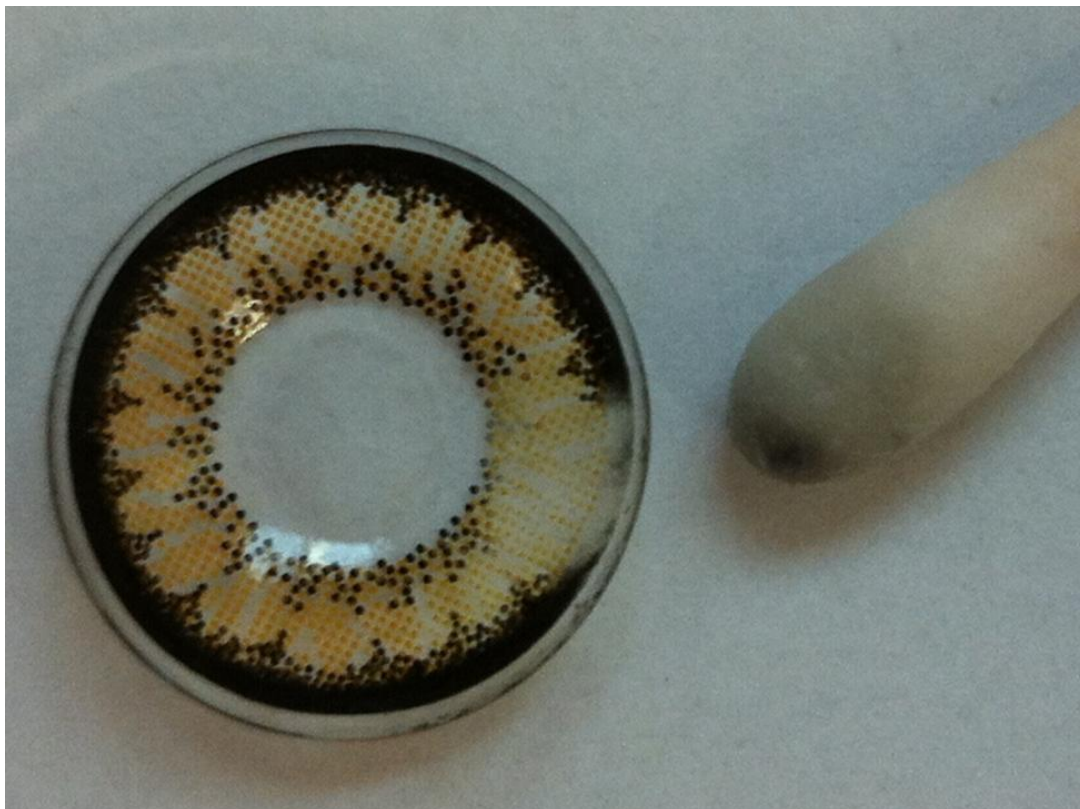
Figure 4.6 Pigments transferred to the wetted cotton bud after rubbing 20 times
