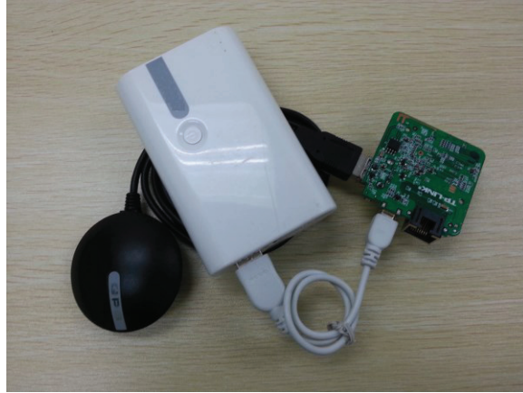
Figure 5.6: Key components in a GPS collection box
