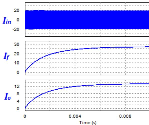
Fig. 5-11 The input current, current after rectifier, output current
