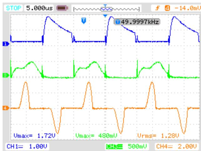
(a) Ch1: inductor current  $i_{Lr3}$ ; Ch3: inductor current  $i_{Lr2}$ ; Ch4:  $i_{Lr1}$
