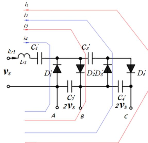
(a) A two stage ac voltage multiplier
