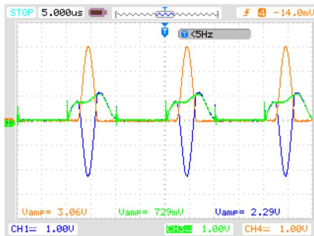
(d) Ch1: current flowing through  $C_4'$ ; Ch3: inductor current  $i_{Lr2}$ ; Ch4: current flowing through  $D_4'$
