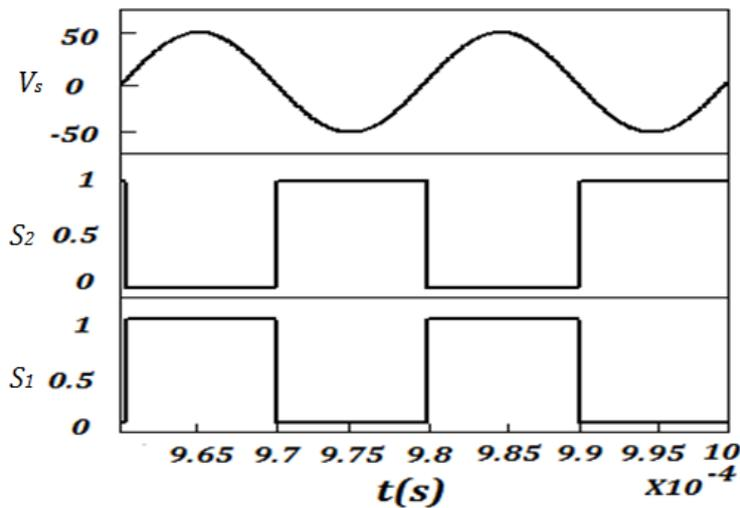
Fig. 3-1 (c) The source voltage and the driving signal
