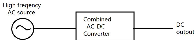
(b) Combined circuit for AC-DC converter
