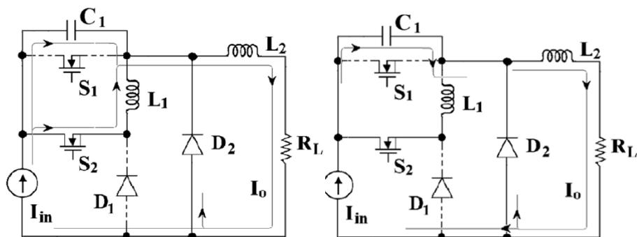
(a) State I:  $S_2$  on and  $S_1$  off (b) State II: freewheeling stage ( $S_2$  on and  $S_1$  off)
