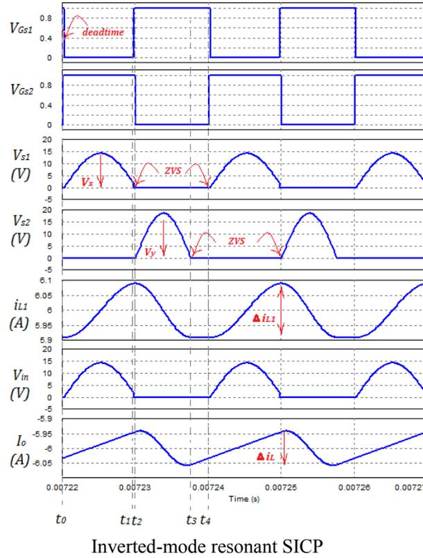
Inverted-mode resonant SICP
