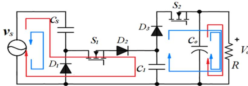
Fig. 3-1 (a) The ac voltage doubler
