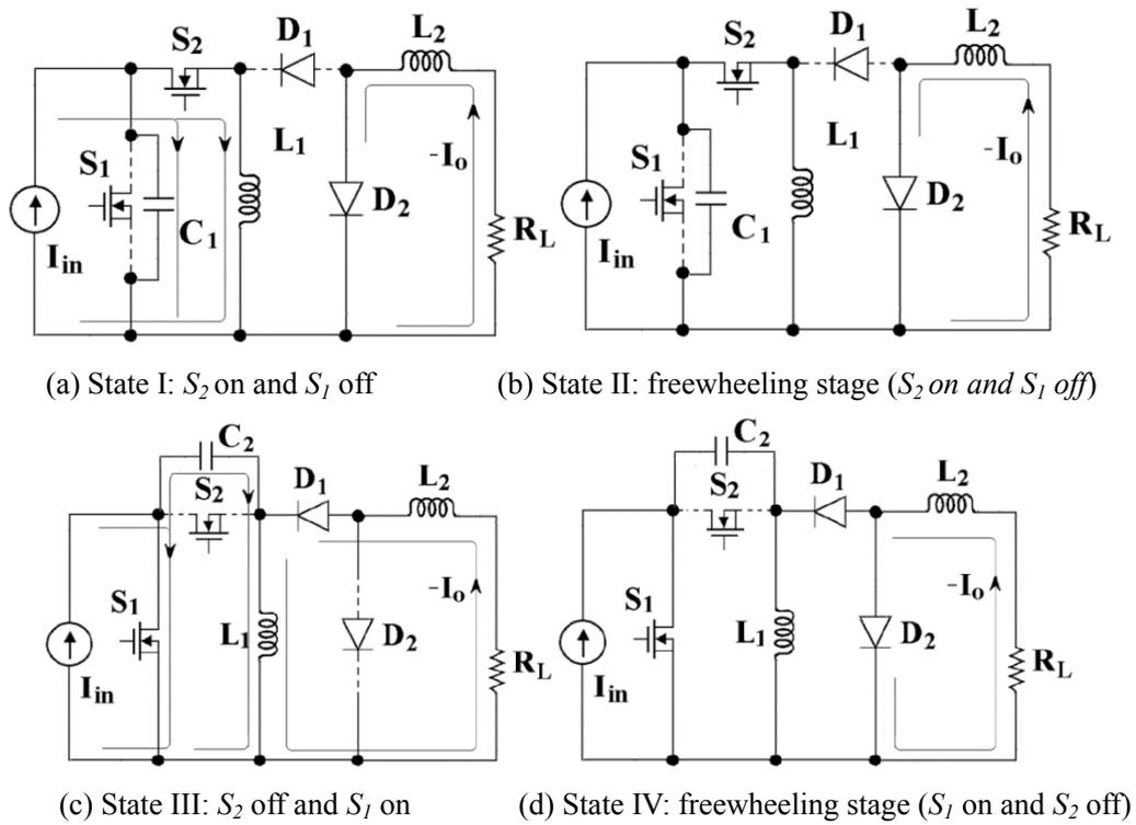
Fig. 5-6 The four operation states of inverted-mode resonant SIPC
