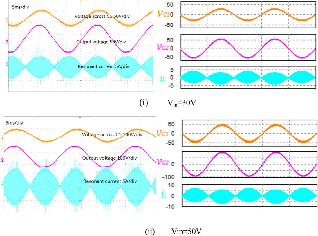
Fig.2-7 The performance of the proposed topology with different input voltages, when  $R=47\Omega$ ,  $L_r=1.2\mu H$ ,  $C_1=C_2=2.2\mu F$  (left: experiment, right: simulation)
