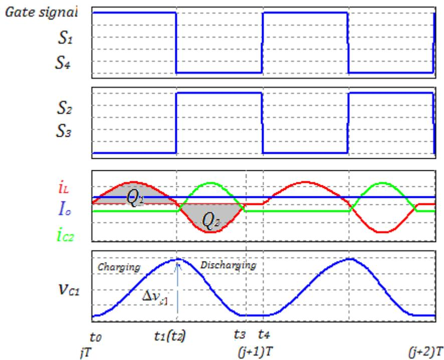
(c) Waveforms of the circuit in steady state.
