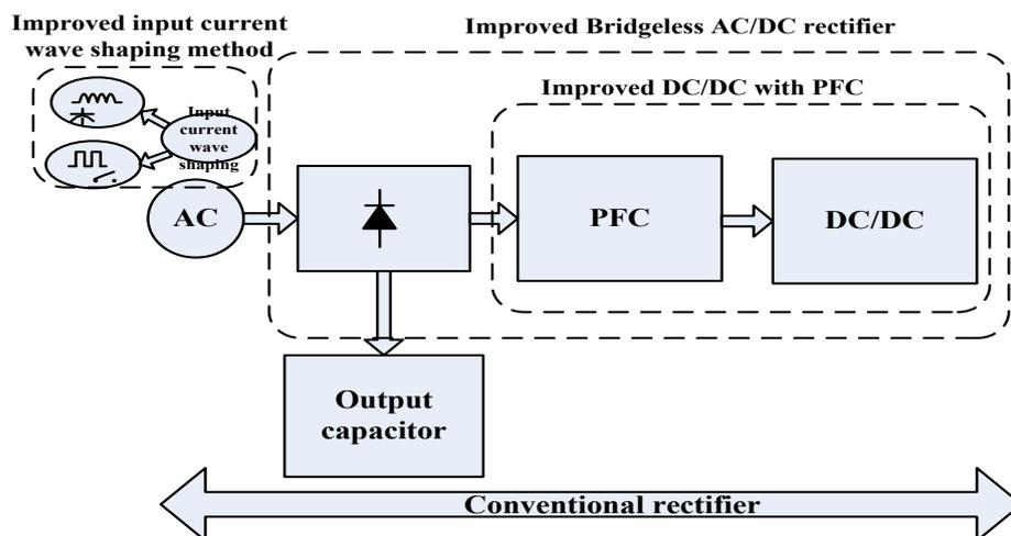
Fig. 1-3 The conventional AC/DC conversion and the improved solutions
