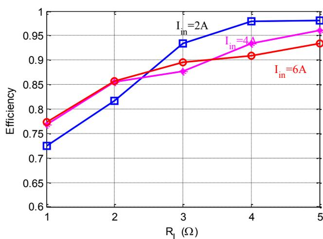
(b) Measured efficiency versus load
