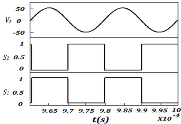
(a) The source voltage and the driving signal
