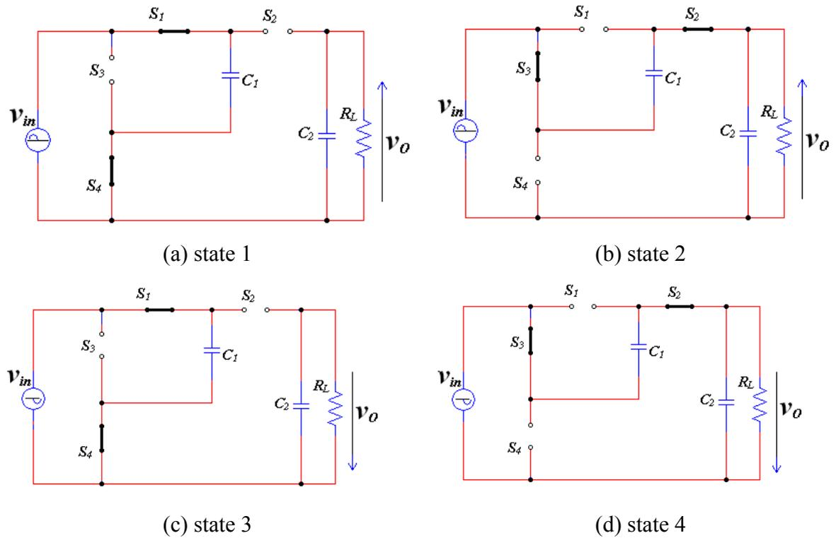
Fig. 2-2 Operational states of the ac-ac step-up switched capacitor power converter without resonant inductor
