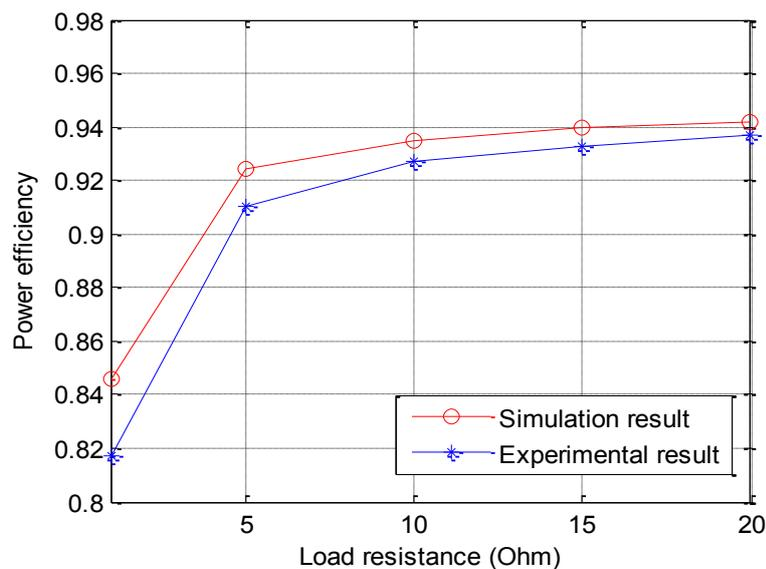
Fig. 3-13 Power efficiency versus load resistance
