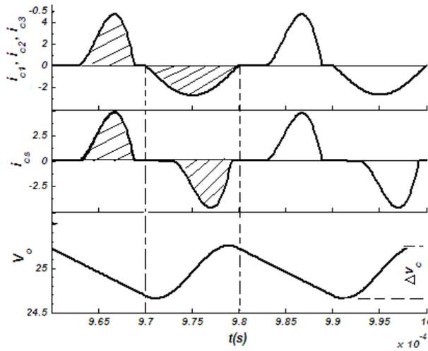
Fig. 3-6 The waveform of current  $i_{cs}$ ,  $i_c$  and the output voltage  $V_o$
