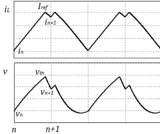
Fig. 7-2 the stroboscopic map of the inductor current and output
