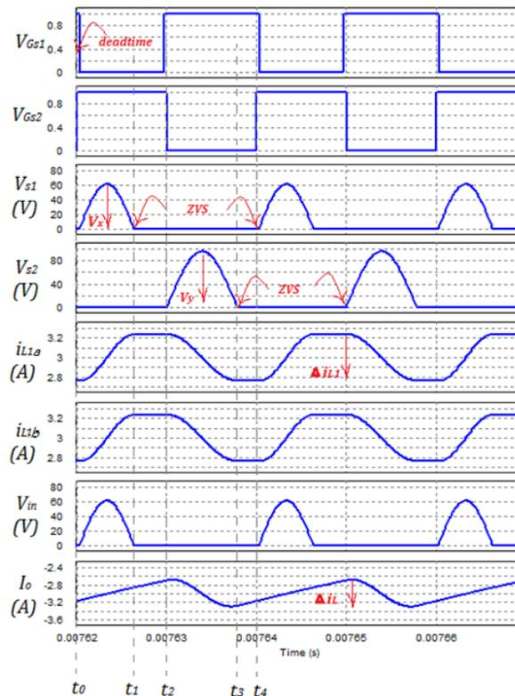
Fig. 6-9 Simulation waveform of -1/2-mode resonant SICP ( $L_{1a}=L_{1b}=500\mu\text{H}$ ,  $f_s=50\text{ kHz}$ ,  $I_{in}=6\text{A}$ )
