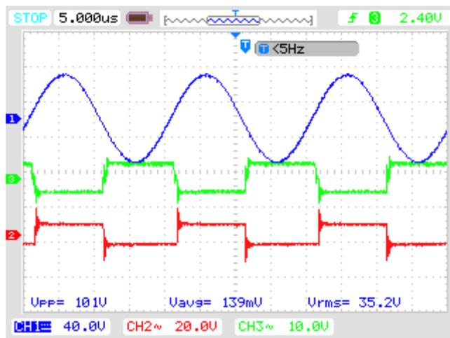
(a) Ch1: input voltage; Ch2: switched signal S1; Ch3: switched signal S2
