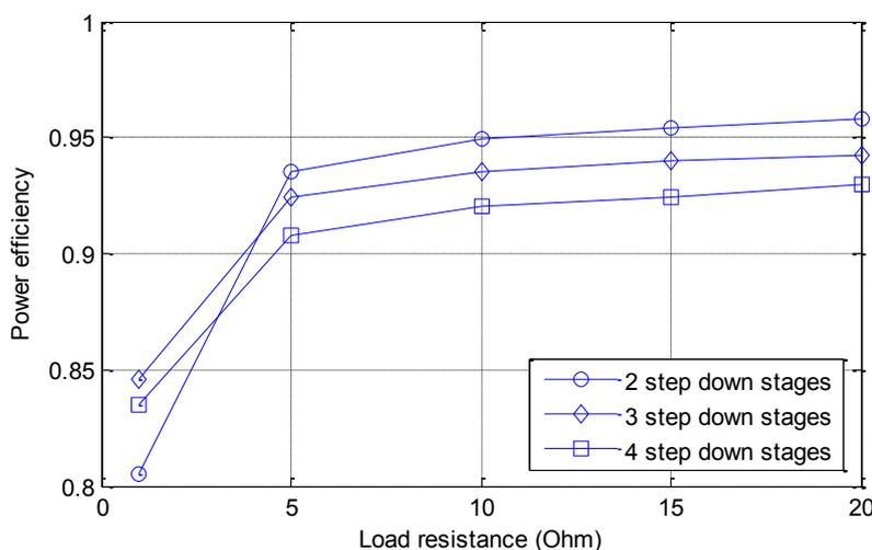
(b) Power efficiency versus load resistance in different step down stages
