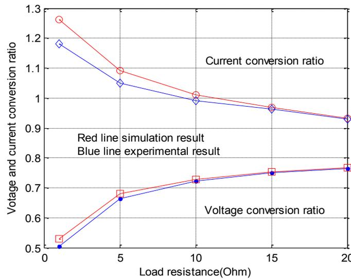
Fig. 3-11 Voltage and current conversion ratios versus load resistance
