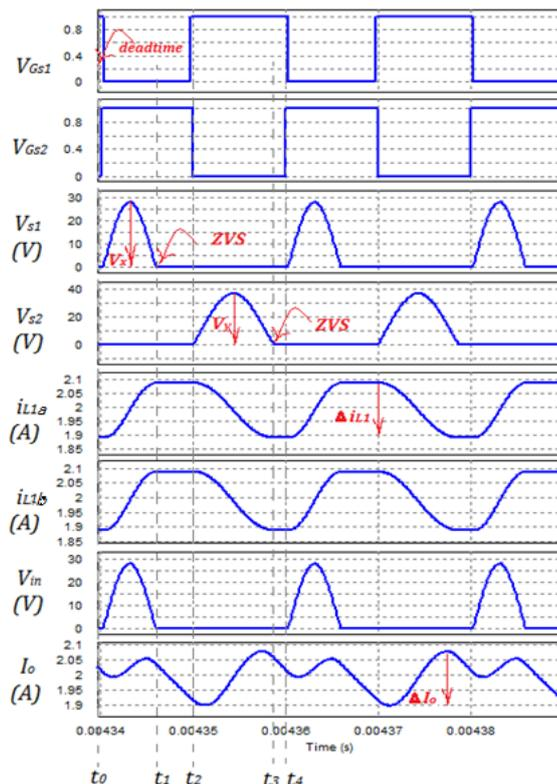
Fig. 6-7 Simulation waveform of 1/3-mode resonant SICP ( $L_{1a}=L_{1b}=500\mu\text{H}$ ,  $f_s=50\text{ kHz}$ ,  $I_{in}=6\text{A}$ )
