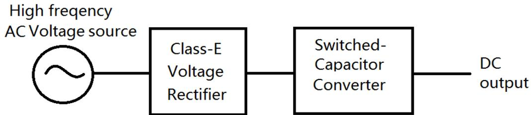
(a) Cascaded of Class-E voltage rectifier with switched-capacitor converter
