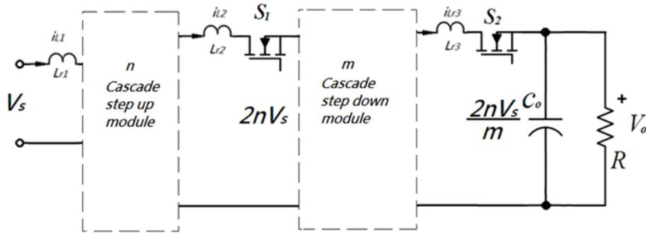
Fig. 4-1 Block diagram of the proposed circuit
