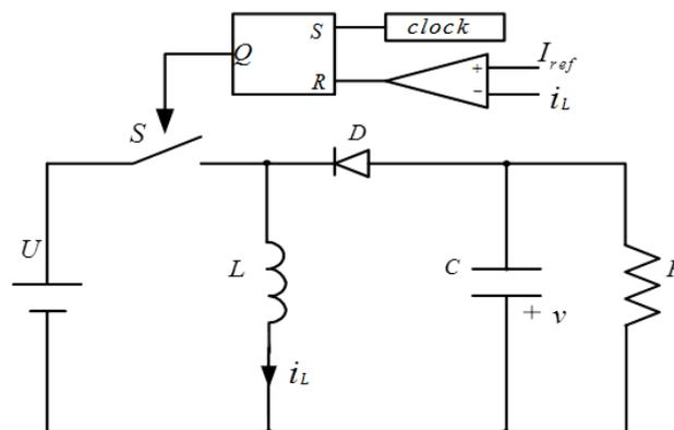
Fig. 7-1 Peak current mode control of Buck-boost converter
