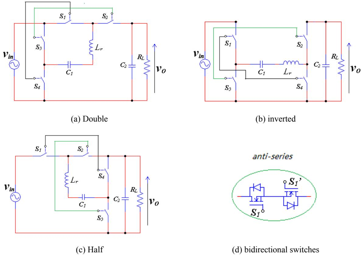
Fig.2-1 The family of proposed ac-ac switched capacitor power converter and switches
