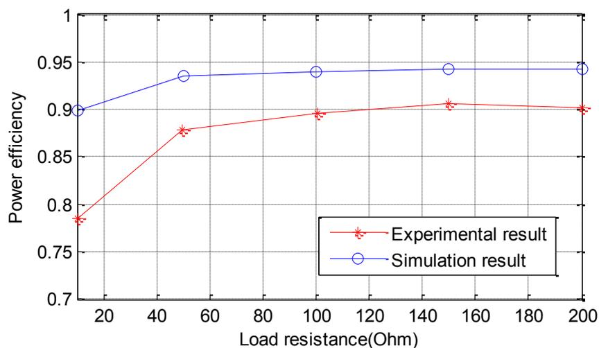
(a) Simulation and experimental result of power efficiency
