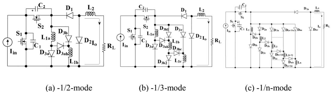
Fig. 6-5 Proposed inverting resonant step down switched-inductor converters
