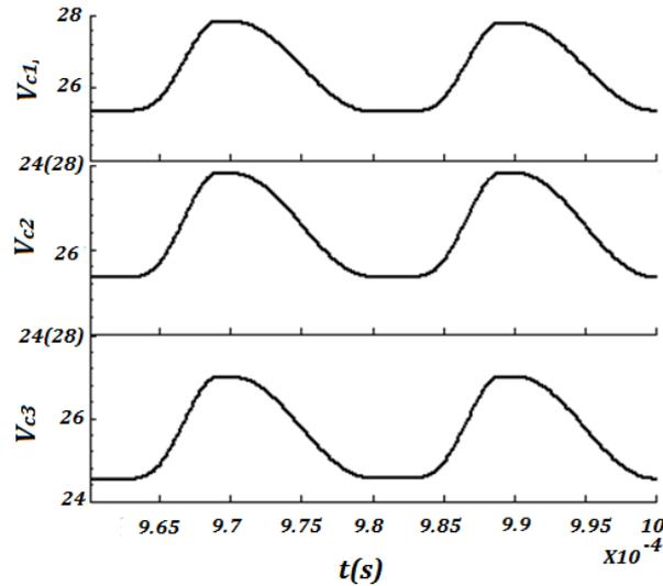
Fig. 3-4 (c) The voltage across capacitor  $C_1$ ,  $C_2$  and  $C_3$
