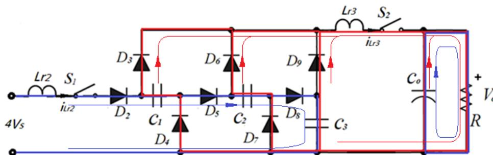
Fig. 4-5 (a) Three stages step down converter
