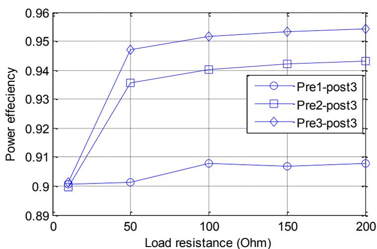
(c) The power efficiency versus output current of 1, 2, 3 pre-stage, 3 post-stage.
