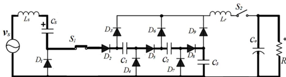
Fig. 3-3 (b) The operation states working in positive half wave ( $S_1$  is on and  $S_2$  is off).
