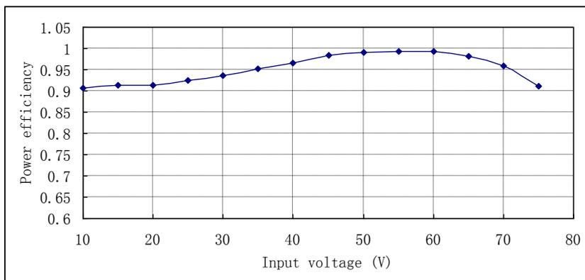
(a) power efficiency versus input voltage
