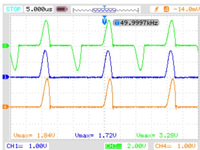
(c) Ch1: current flowing through D4'; Ch3: inductor current  $i_{Lr1}$ ; Ch4: current flowing through D2'
