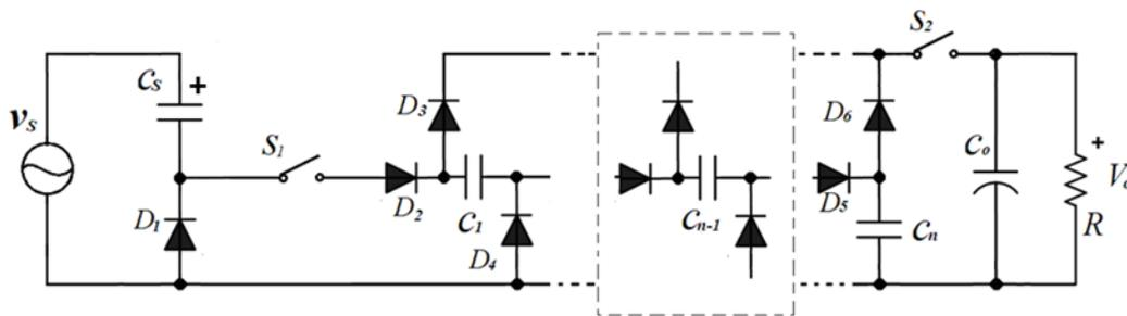
Fig. 3-2 Proposed circuit consisting cascaded SC elements to step down the voltage
