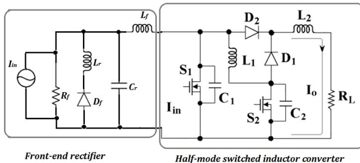
Fig. 5-10 A class-E rectifier with a Half-mode switched inductor power converter
