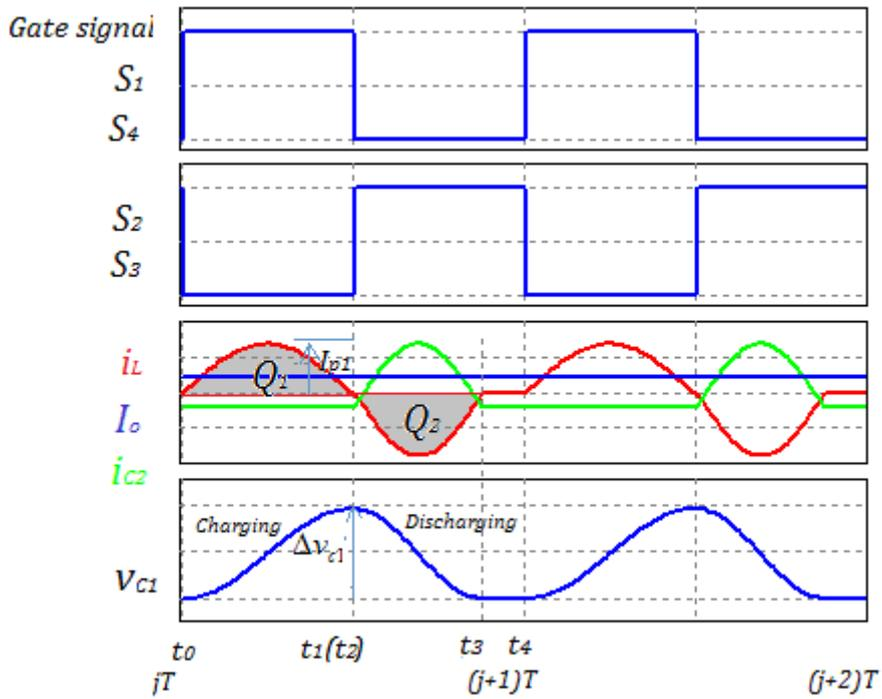
Fig. 2-4. The circuit system, equivalent circuit system and the waveforms of the circuit
