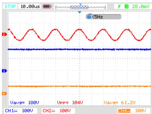
(b) Ch1: stepped up voltage Vo1; Ch2: input voltage; Ch4: output voltage
