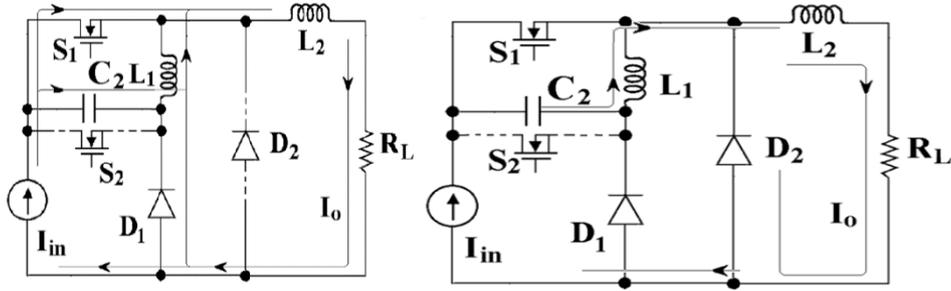
(c) State III:  $S_2$  off and  $S_1$  on      (d) State IV: freewheeling stage ( $S_2$  off and  $S_1$  on)
