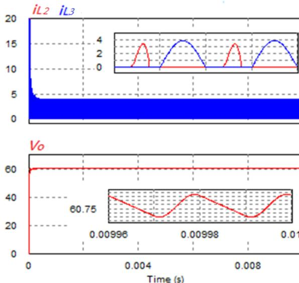
Fig. 4-5(b) The current of resonant inductor and the output voltage
