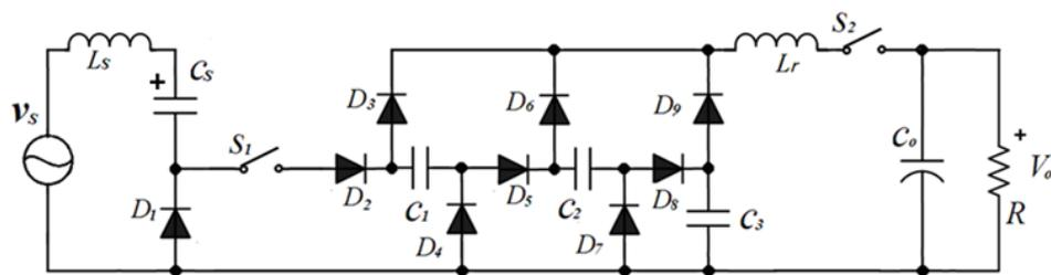
Fig. 3-3 (a) The proposed circuit consisting three cascaded step down SC elements
