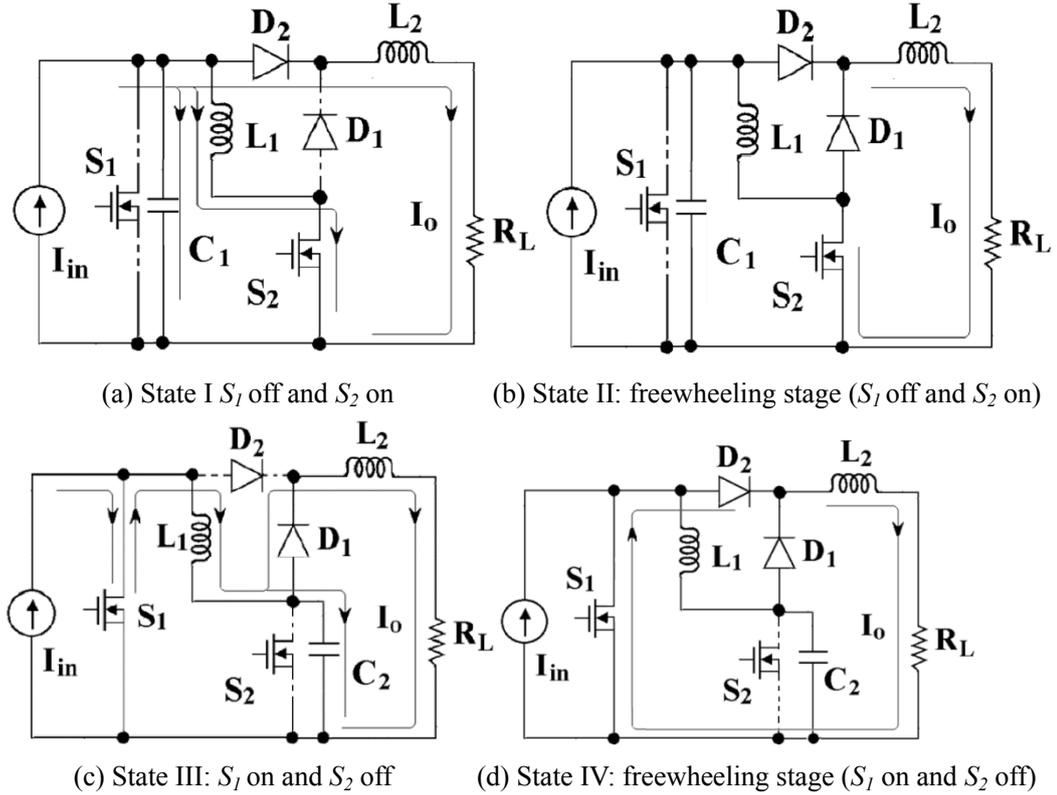
Fig. 5-4 The four operation states of half-mode resonant SIPC
