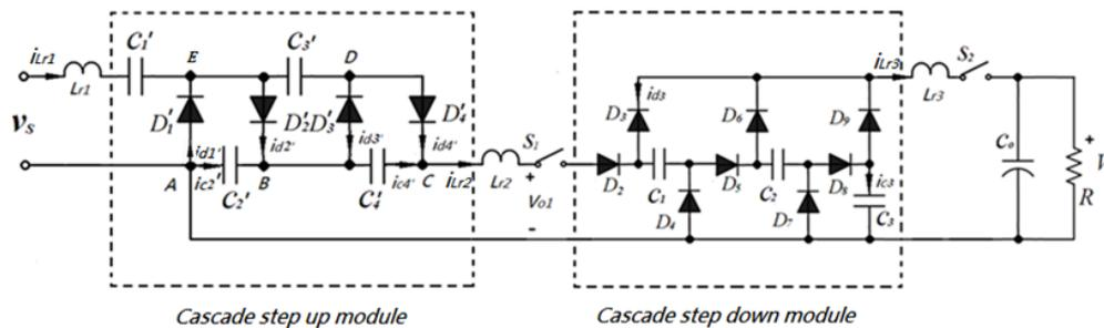
Fig. 4-3 A two step up cells, three step down cells switched capacitor ac/dc converter
