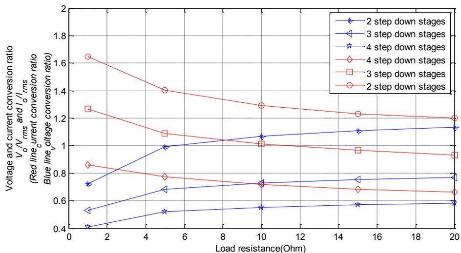
(c) Current and voltage conversion ratio versus load resistance in different step down stages.
