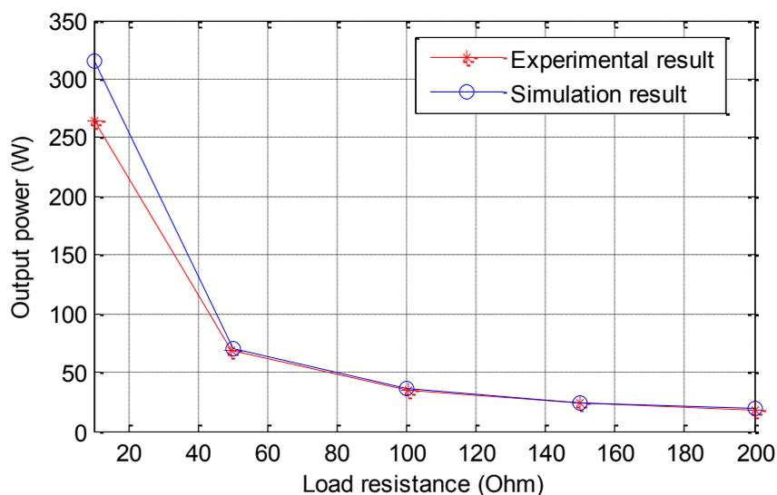
(b) Simulation and experimental result of output power
