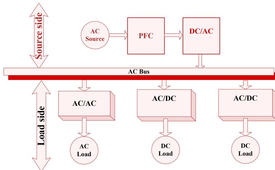
Fig. 1-2 Typical high frequency AC distribution power system architecture.
