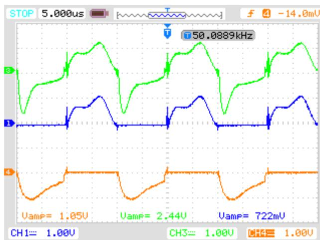
(b) Ch1: inductor current  $i_{Lr2}$ ; Ch3: current flowing through C3; Ch4: current flowing through D3
