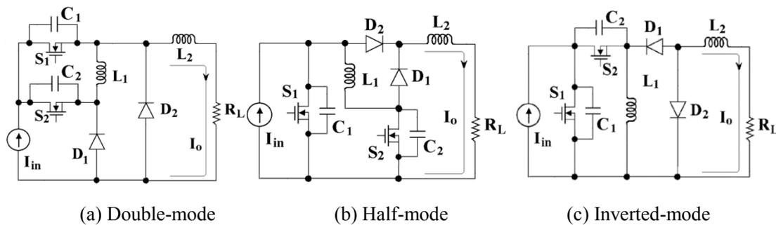
Fig.5-1 Resonant switched-inductor converters
