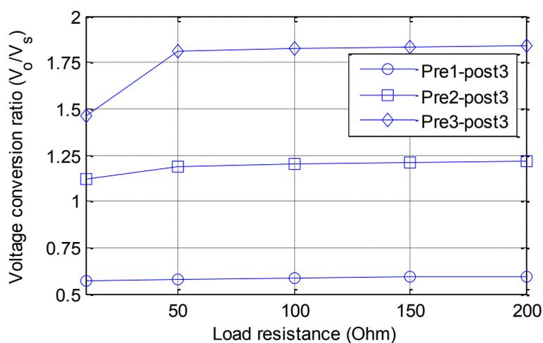
(b) conversion ratio versus load resistance
