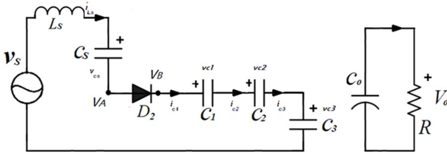
Fig. 3-5 (a) The operation of mode A
