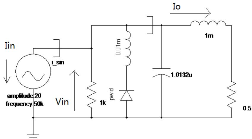
Fig 1-6 Schematic diagram of the Class-E rectifier under current mode
