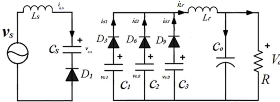
Fig. 3-5 (b) The operation of mode B
