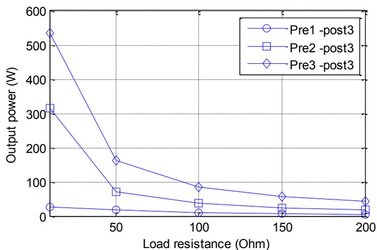
(a) The output power versus load resistance
