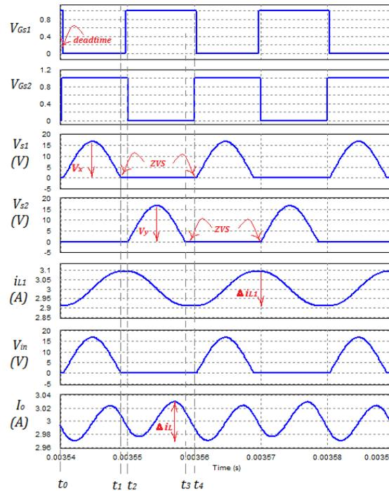
Fig. 5-5 Simulation result of the three resonant SIPC ( $L_1=L_2=500\mu\text{H}$ ,  $f_s=50\text{ kHz}$ ,  $I_m=6\text{A}$ )
