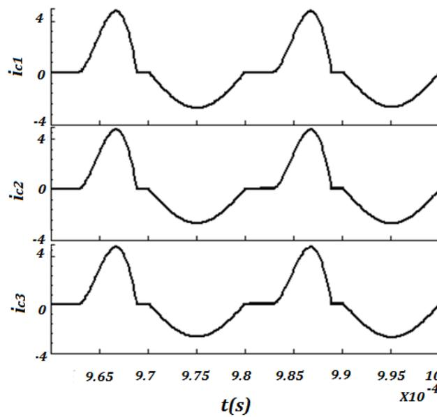
Fig. 3-4 (b) The current flowing through capacitors  $C_1$ ,  $C_2$  and  $C_3$
