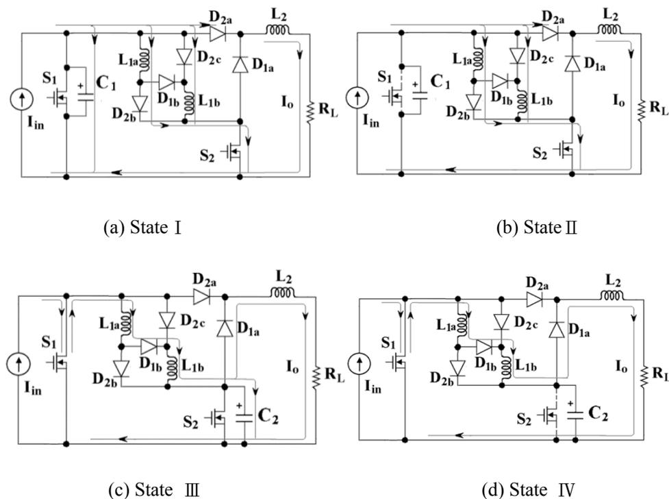
Fig. 6-6 The operation states of 1/3-mode resonant SIPC
