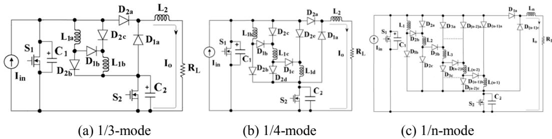
Fig. 6-4 Proposed non-inverting resonant step down switched-inductor converters
