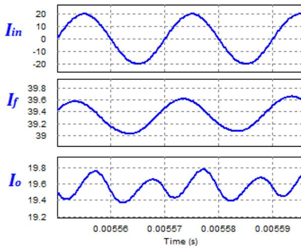
Fig. 5-12 Zoom in of input current, current after rectifier, output current
