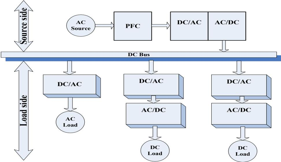
Fig. 1-1 Typical DC distribution power system architecture.
