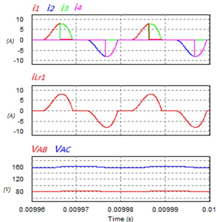
(b) The current and voltage of a two step up cells module
