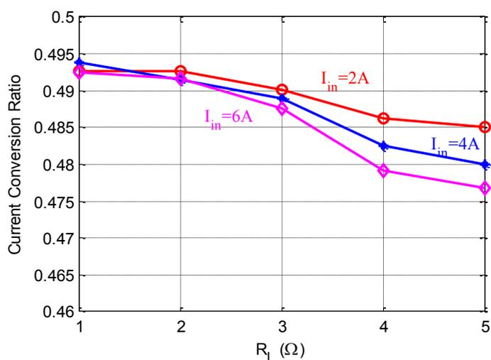
(a) Current ratio versus load
