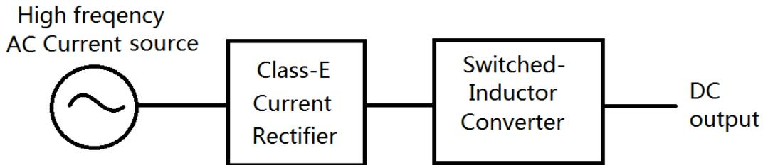
(b) Cascaded of Class-E current rectifier with switched-inductor converter
