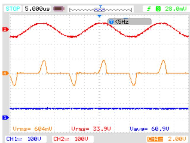
(c) Ch1: output voltage; Ch2: input voltage; Ch4: input current
