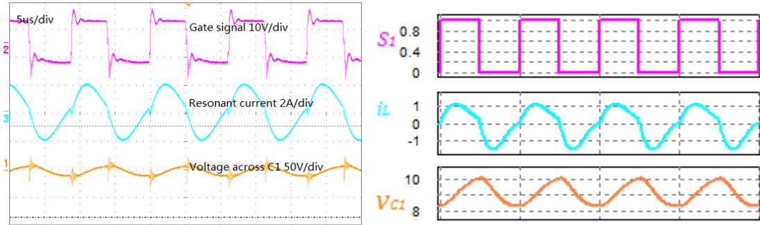
(b) The gate signal, resonant current, voltage across  $C_1$  when  $R=47\Omega$
