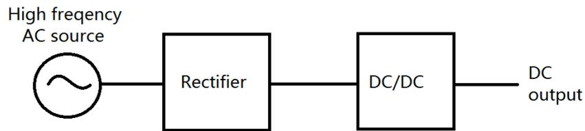
(a) Separate rectifier and DC/DC converter
