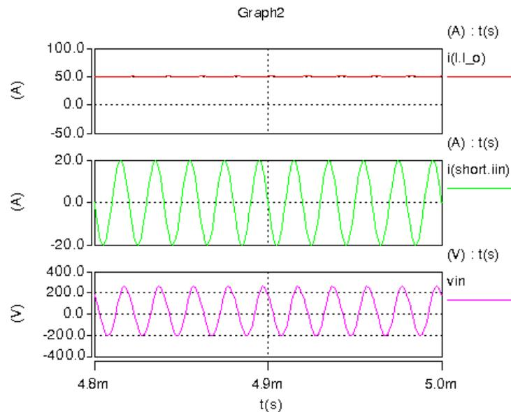
Fig 1-7 The simulated waveforms of the Class-E rectifier
