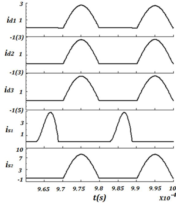
Fig. 3-7 The current flowing through the diodes and switches
