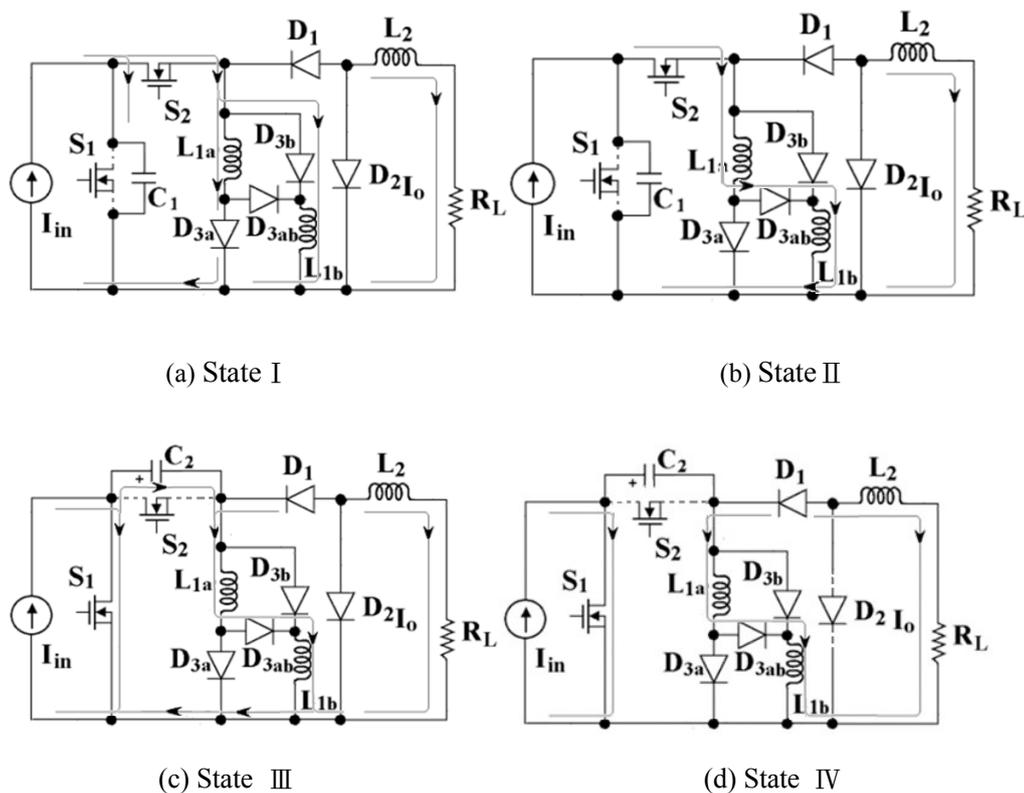
Fig. 6-8 The operation states of -1/2 -mode resonant SIPC
