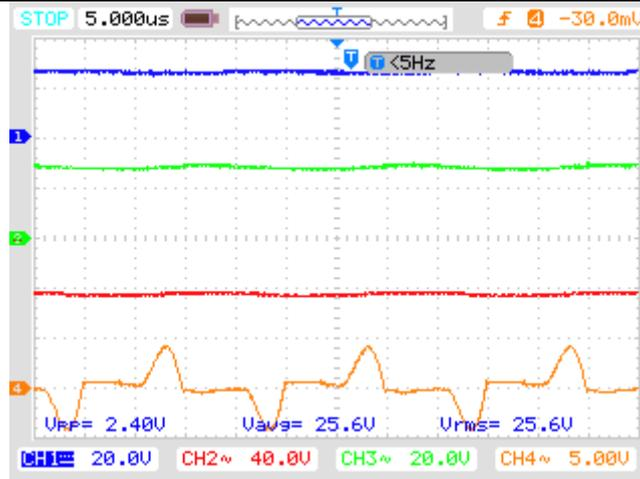
(c) The voltage across capacitors  $C_s$  and  $C_1$  and the output voltage  $V_o$  and current flowing through  $L_s$  (Ch1:  $V_o$ ; Ch2:  $V_{cs}$ ; Ch3:  $V_{c1}$ ; Ch4:  $i_{Ls}$ )
