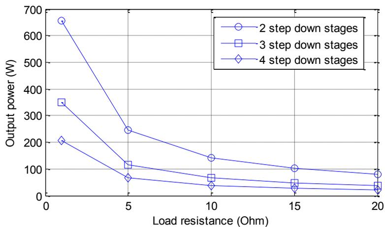
(a) Output power versus load resistance in different step down stages
