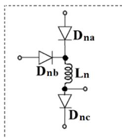
Fig. 6-3 Proposed switching inductor cell
