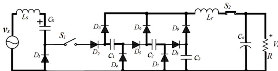
Fig. 3-3 (c) The operation states working in negative half wave ( $S_1$  is off and  $S_2$  is on).
