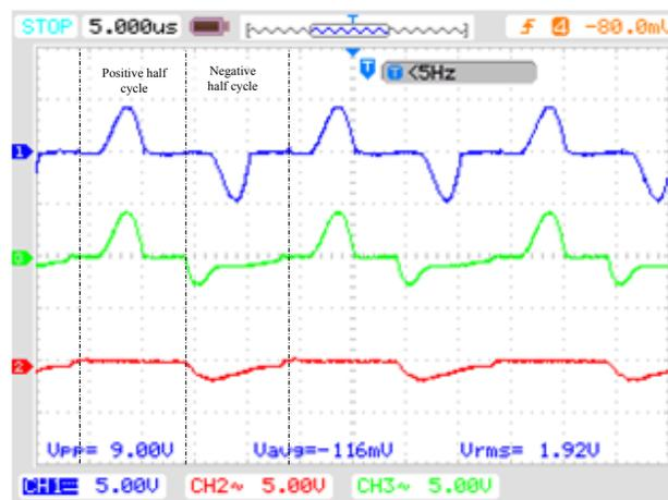
(b) The current following through capacitors  $C_s$ ,  $C_1$ , and  $D_3$
