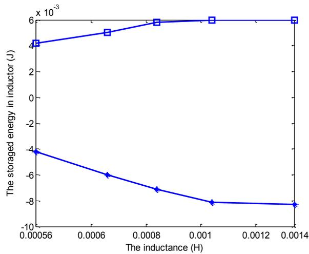
Fig. 7-22 Experimental result of boundary for storage energy in inductor
