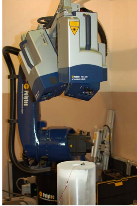
Figure 3.17: Position of the scanner heads for the ‘top view’ propagation measurements.
