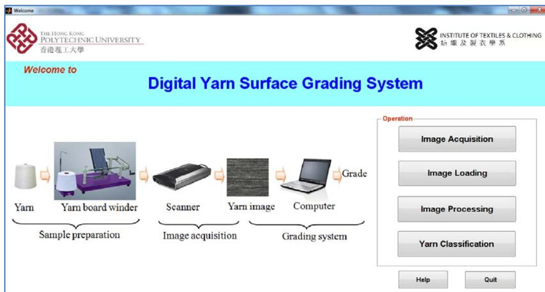
Figure 5.34 Main interface of the digital yarn grading system.
