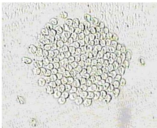
Figure 2.16 Cross-sectional image of a high-twist ring spun yarn (Tencel) [32].
