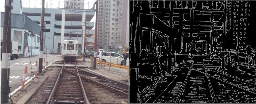
Figure 2-9 Original image and extracted edge map
