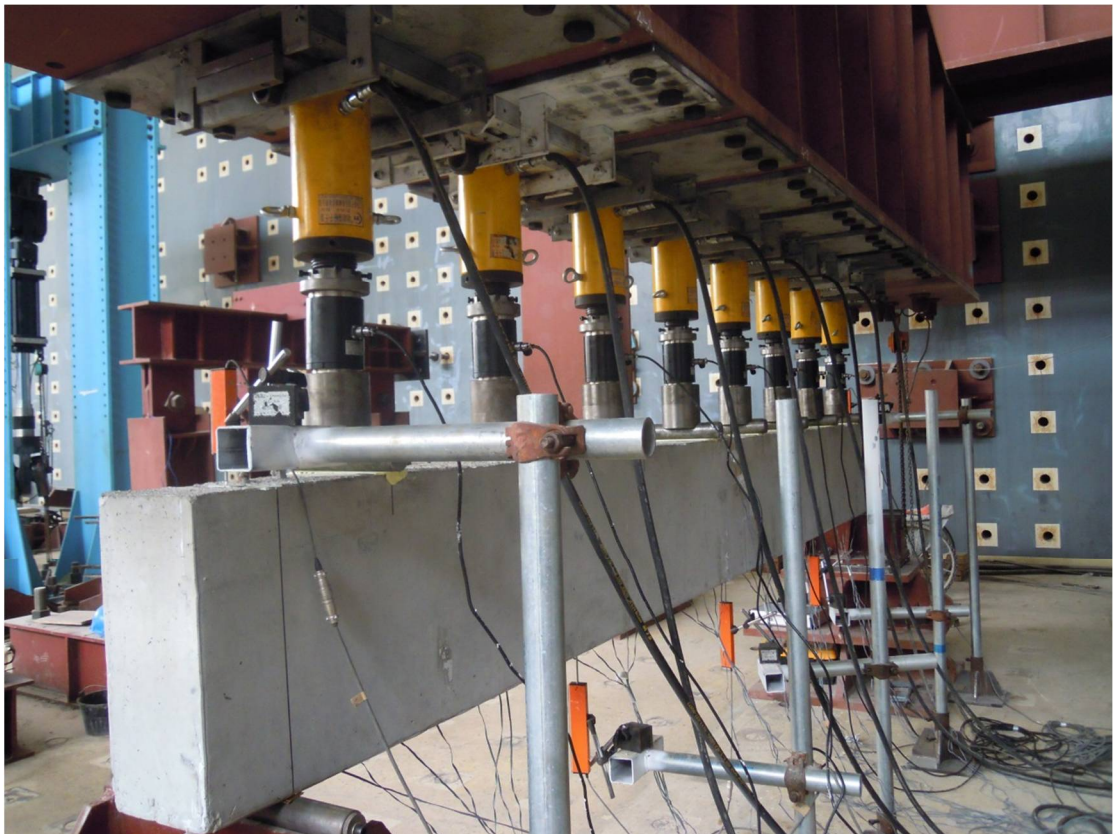
Figure 3.8 Installation of LVDTs
