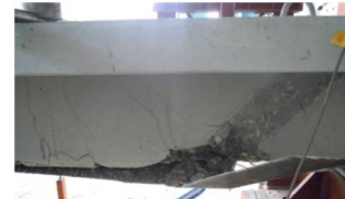
Figure 7.16 Failure modes of specimens with inclined FRP U-jackets in Series-I
