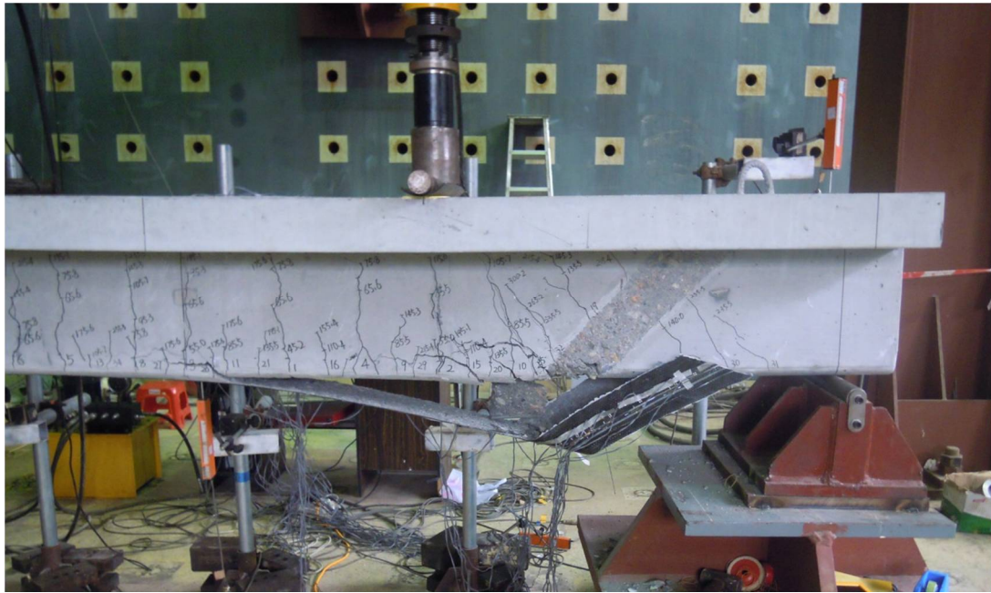
Figure 7.22 Failure mode of Specimen I1L1W120b
