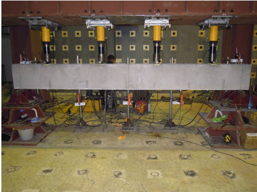
(a) Specimen LP4SP1000 under four-point loading
