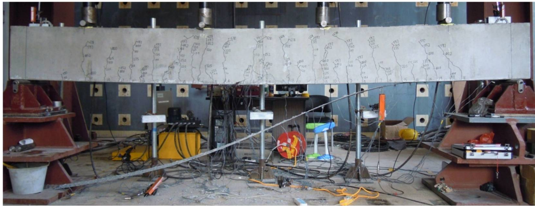
(d1) Failure mode of Specimen LP4SP1000
