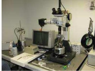
*Figure 2-10. Atomic force microscopy*
