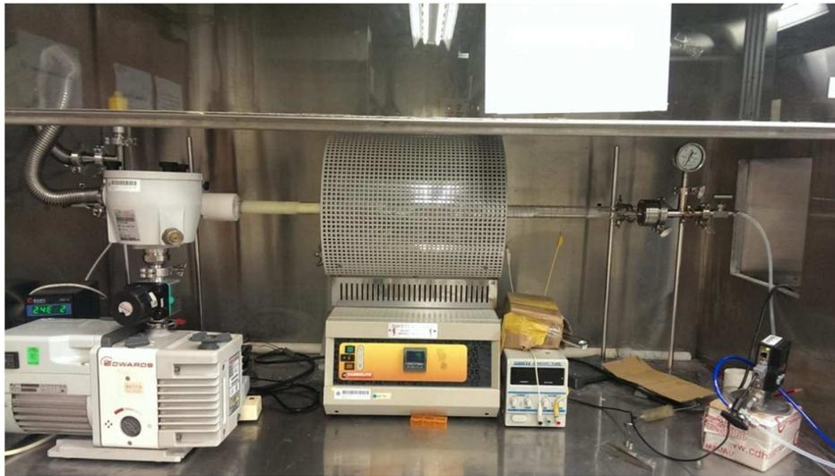
Figure 2-2. The experimental setup of vapor phase deposition.
