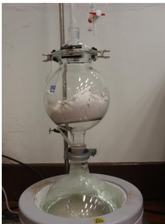
Figure 4. 2 Steam distillation apparatus.
