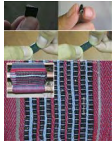
Figure 2-11: Charging-up Smart Fabrics with Woven Battery
