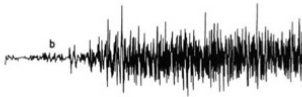
Figure 2-37: Acoustic emission waveforms detected by continuous type piezoelectric transducers
