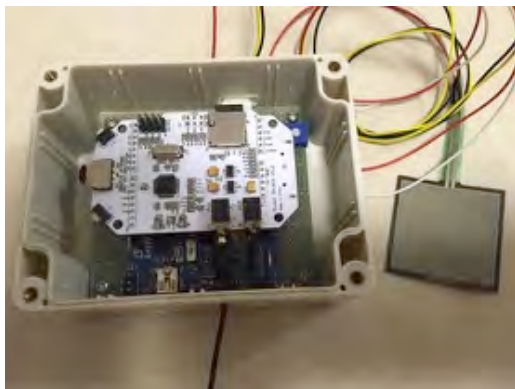
Figure 4-13: The developed pressure sensor
