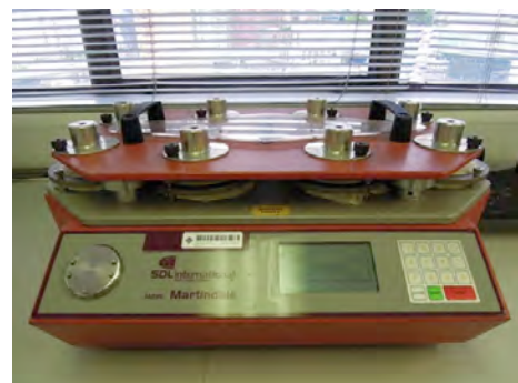
Figure 5-1: Abrasion Test Machine
