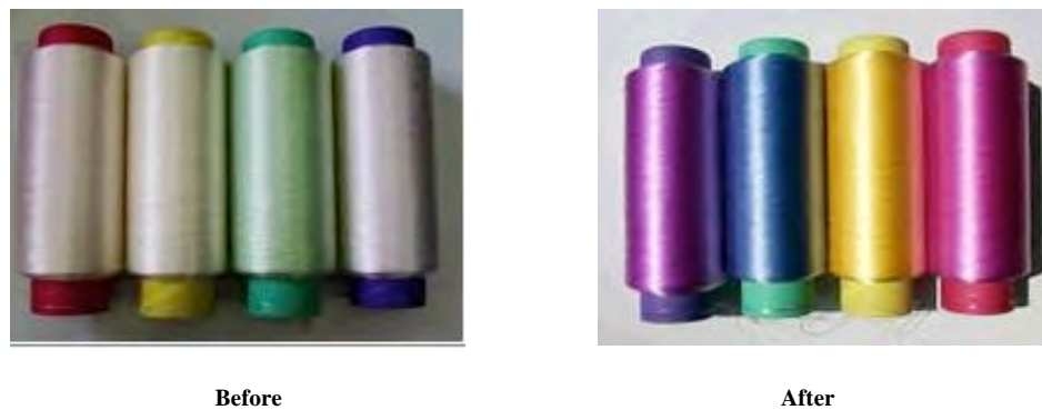
Figure 2-33: Before and after: Colour-changing yarn using Photochromic material
