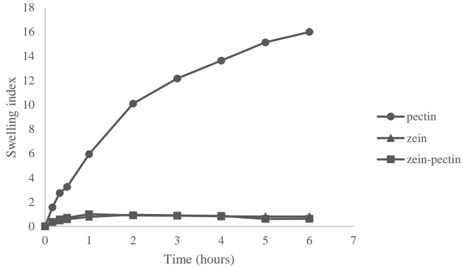
Figure 4.5 Swelling test of zein, pectin and zein-pectin films. The film samples were incubated in phosphate buffer solution of pH 7.4 at 37 °C. For easy measurement, pectin film was cross-linked by 50 mM calcium chloride to reduce the solubility in water.
