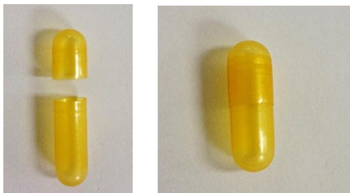
Figure 3.12 A two-piece zein hard capsule of size #0 plasticized with oleic acid.
