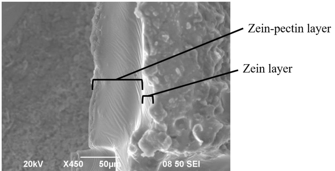
Figure 4.3 SEM images of the cross section of one layer zein-pectin and one layer zein.
