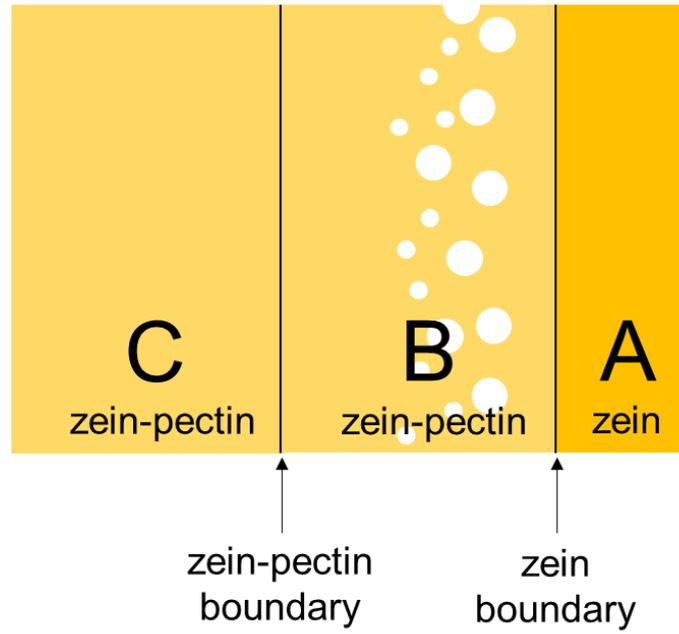
Figure 4.4 Schematic diagram of the three-layered structure of zein-pectin coated dosage form for colon-specific drug delivery. (A) The zein layer formed from 20% (w/v) zein solution. (B) The zein-pectin layer prepared by coating zein solution after pectin, with pores formed. (C) The zein-pectin layer same as layer B, without pores.
