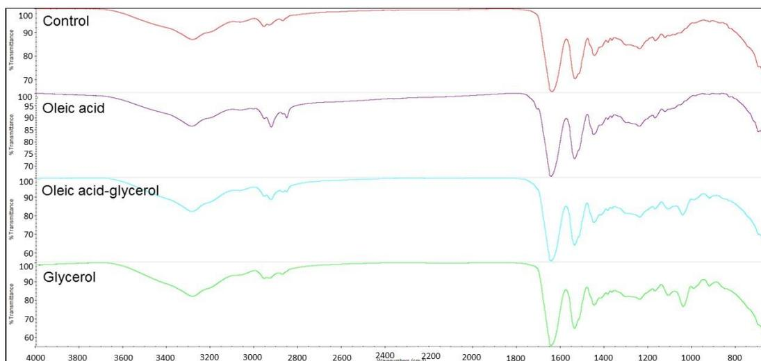
Figure 3.4 FTIR spectra of the oleic acid-plasticized zein films. The total plasticizing levels were 20% weight ratio to zein. Oleic acid-to-glycerol-plasticized at the ratio of 2:1.
