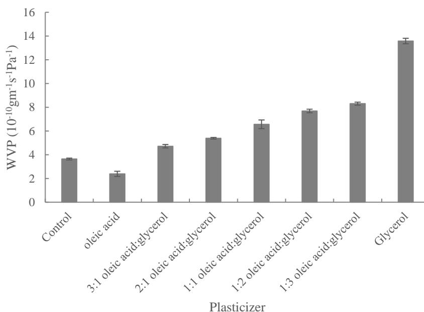
Figure 3.3 WVP of zein films at different ratio of oleic acid to glycerol. Total plasticizer content was 70% to the weight of zein.
