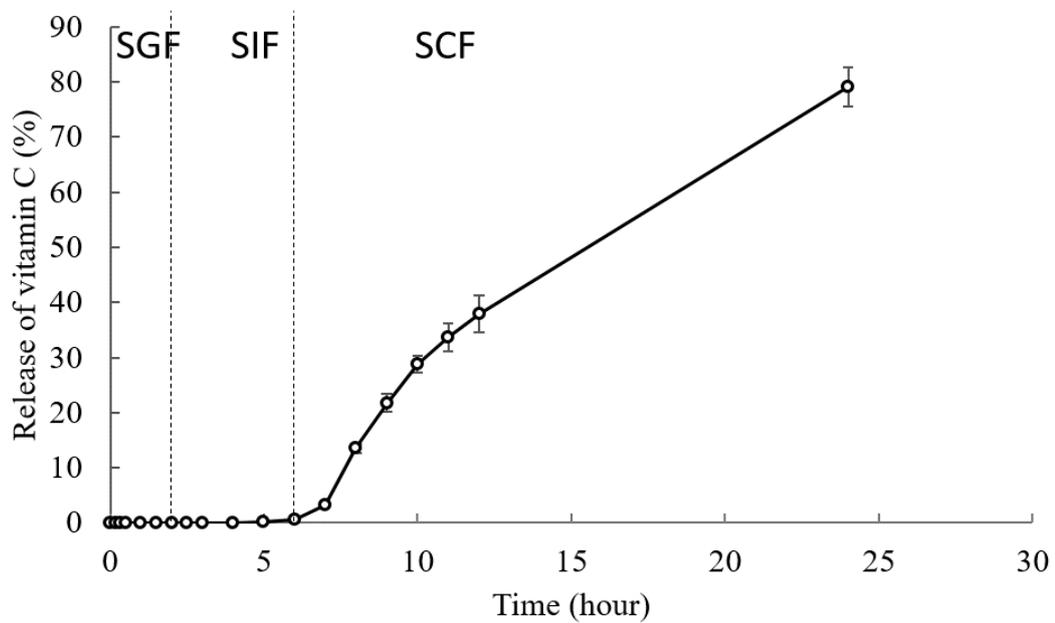
Figure 4.7 Release profile of zein-pectin coated dosage form. The release media were SGF at 0-2 hours, SIF at 2-6 hours and SCF at 6-24 hours.
