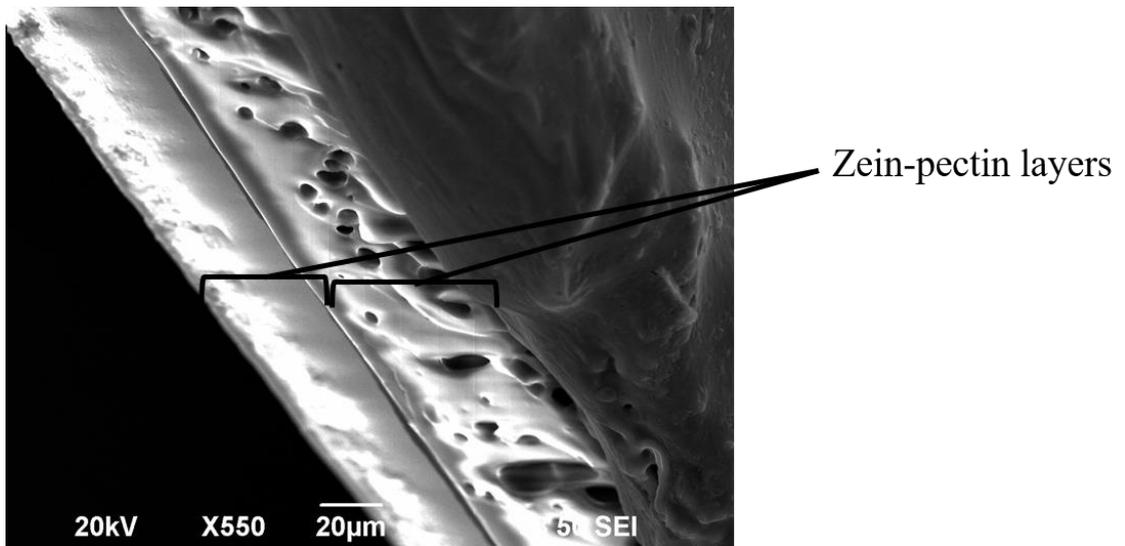
Figure 4.2 SEM images of the cross section of the zein-pectin coated dosage form.
