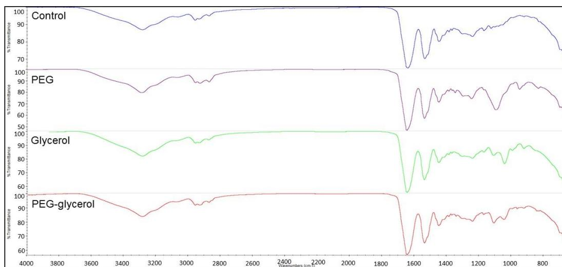
Figure 3.5 FTIR spectra of the PEG-plasticized zein films. The total plasticizing levels were 20% weight ratio to zein. PEG-to-glycerol-plasticized at the ratio of 2:1.
