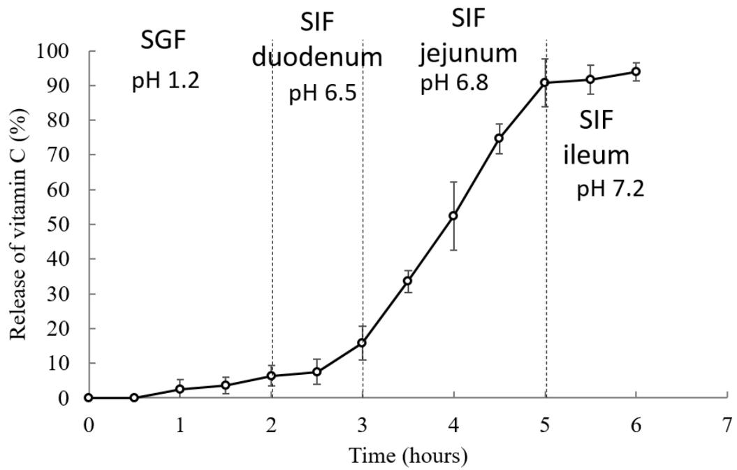
Figure 3.13 Release profile of the oleic acid-plasticized zein capsules. The capsule was incubated in the release media SGF for 2 hours, SIF-duodenum for 1 hour, SIF-jejunum for 2 hours and SIF-ileum for 1 hour.
