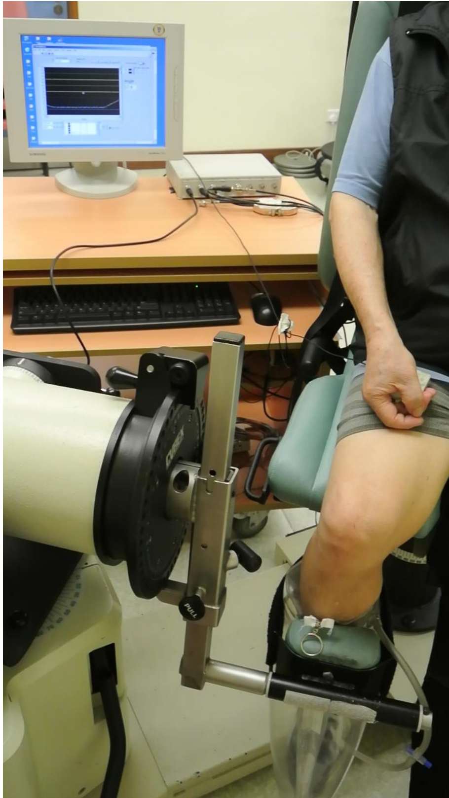
Figure 5: Setup for knee joint position test. A participant was seated on an isokinetic exercise chair with hip at 80^{\circ} of flexion and knee axis aligned with the dynamometer axis of rotation. An inflatable air splint was applied to the lower leg to minimize sensory input.
