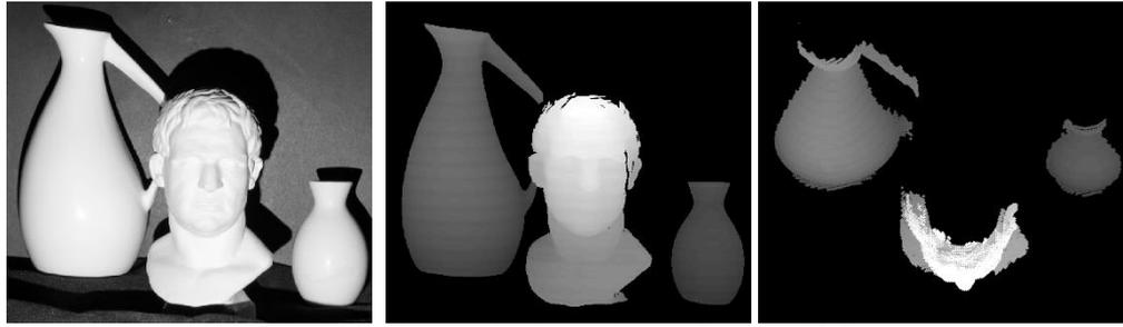
Figure 5-11. A scene of complex objects (the first column). Result of 3-D reconstruction using the proposed algorithm (second column). The top view of 3D reconstruction (the last column).
