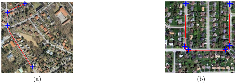
FIGURE 6.6: Comparison with the existing semi-automatic method. (a) The proposed method results which are shown in red. (b) The results produced by Hu et al. (2004) which are shown in red. Seed points are shown with blue crosses.
