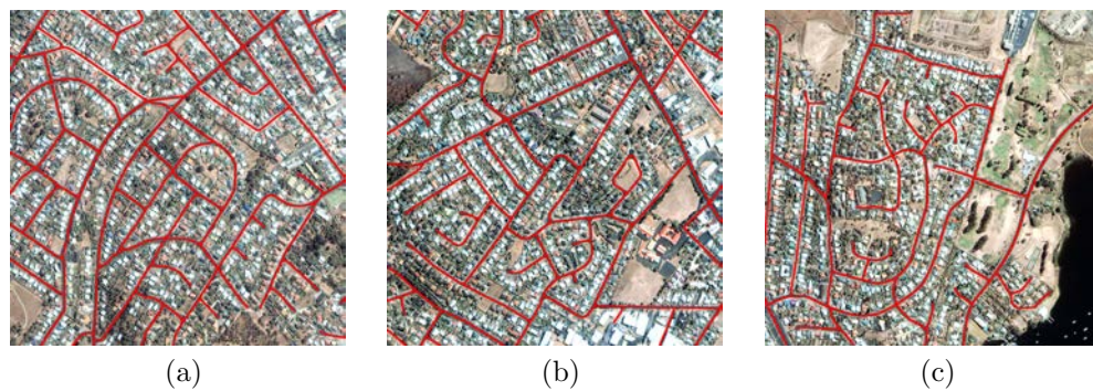
FIGURE 3.10: Road extraction results for three test areas extracted from an Ikonos image of Moonah (Australia).
