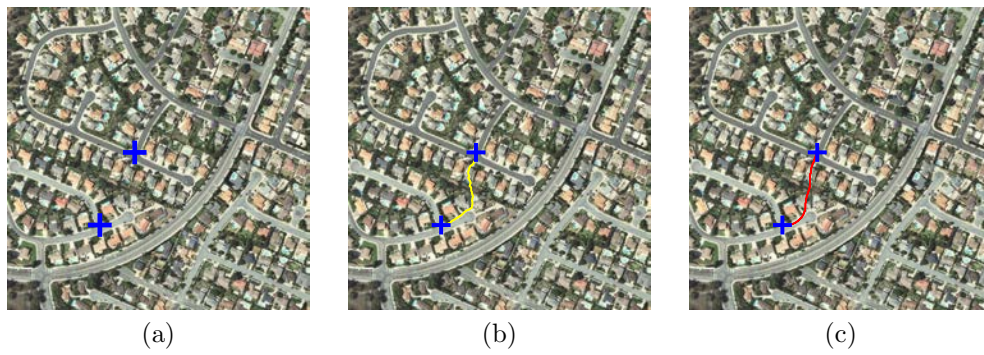
FIGURE 6.5: Results on the third image. (a) Test image in which seed points which are shown in blue cross. (b) The geodesic method result which is shown in yellow. (c) The proposed method result which is shown in red.
