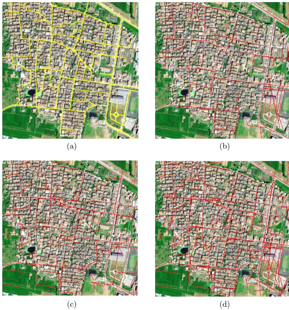
FIGURE 4.10: Comparison of the results of different road extraction strategies on the Xuzhou test area: (a) ground truth; (b) EM results; (c) linearity filter results; (d) fusion result.
