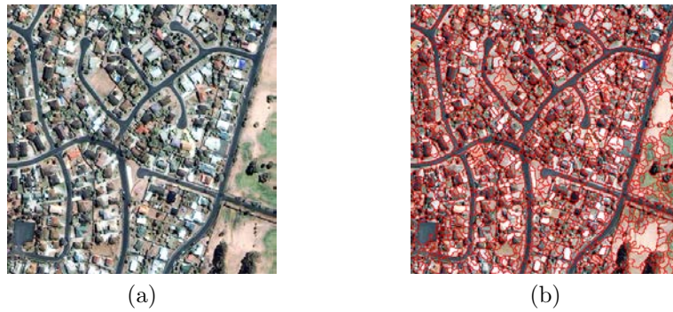
FIGURE 1.7: (a) A test optical satellite image. (b) The derived objects where the boundary between objects is shown in red.
