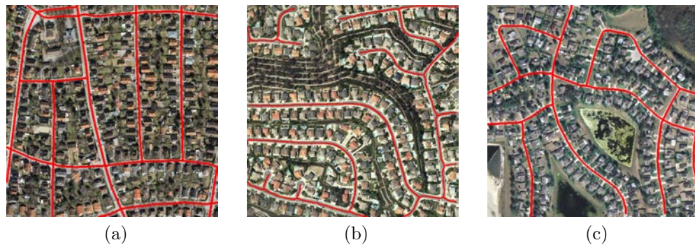
FIGURE 3.9: Road extraction results on three QuickBird test samples (VPLab, 2015): (a)-(c) show the three test areas, respectively.
