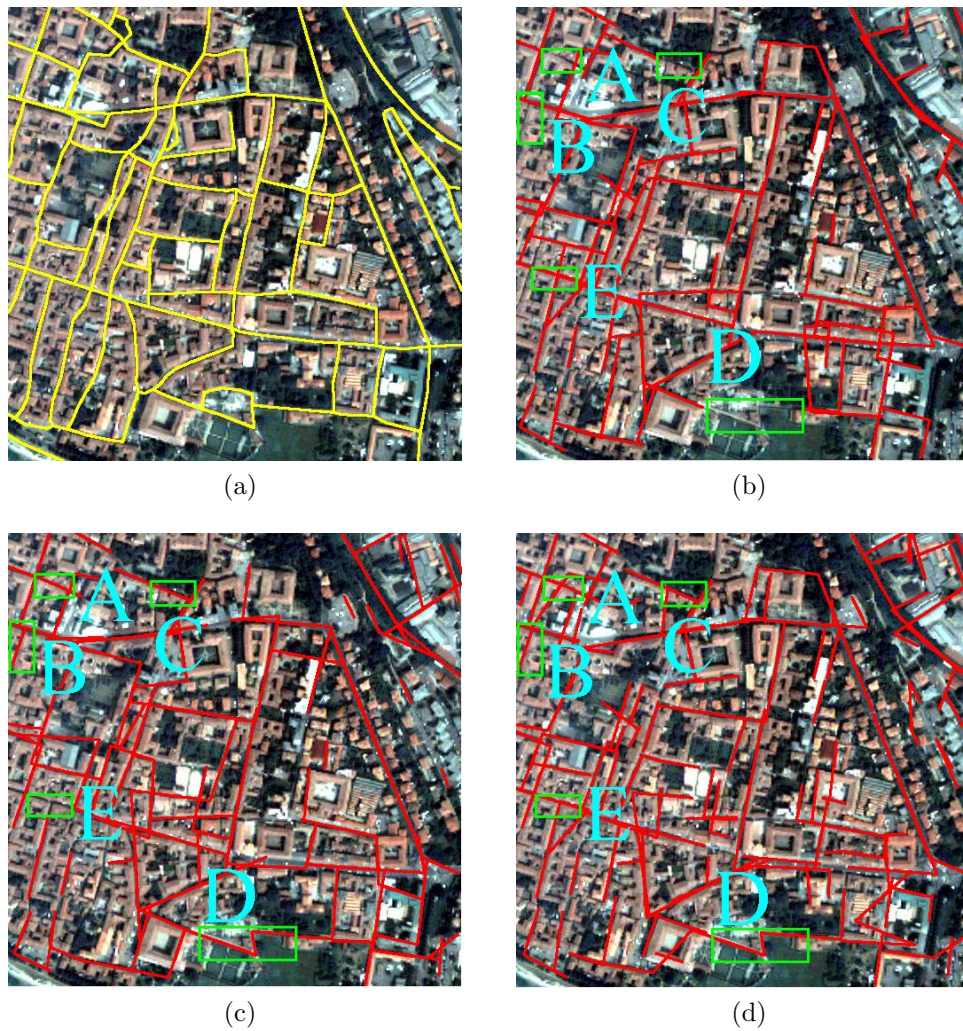
FIGURE 4.9: Comparison results of different road extraction strategies on the Pavia test area: (a) ground truth; (b) EM result; (c) linearness filter result; (d) information fusion result.
