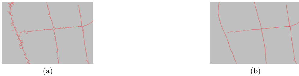
FIGURE 2.15: (a) The thinning algorithm extraction result. (b) The proposed method extraction result.
