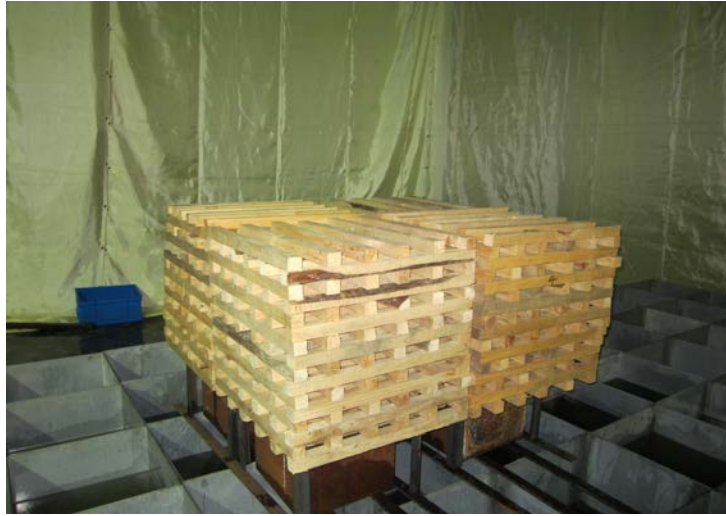
Figure 7.6 Wood crib and water collection pan placement
