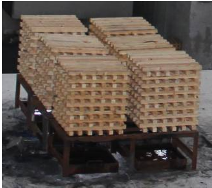
Figure 4.13 W5 wood crib placement
