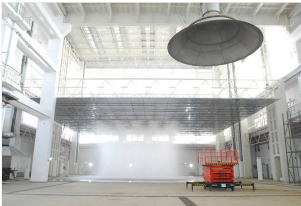
Figure 4.2 10 MW heat calorimeter system
