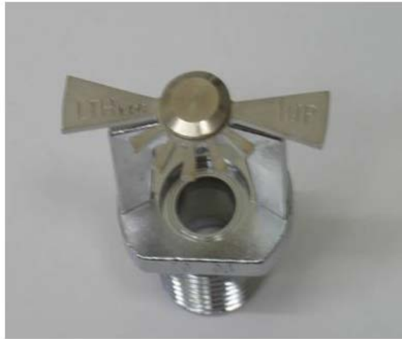
Figure 5.11 Testing sprinkler head
