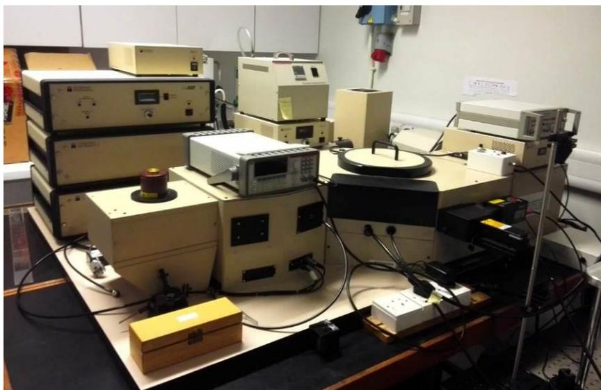
Figure 2.6 Photography of Edinburgh FLSP920 spectrometer used in our laboratory.
