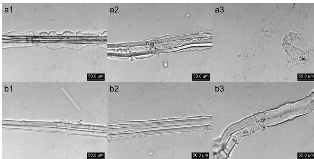
Figure 6.5 Optical microscope images of dissolution in 9.3 M LiBr of (a) CS and (b) TrialS under (1) immersion, (2) after immersion for 60 min, and (3) after heating for 60 min at 65 °C.
