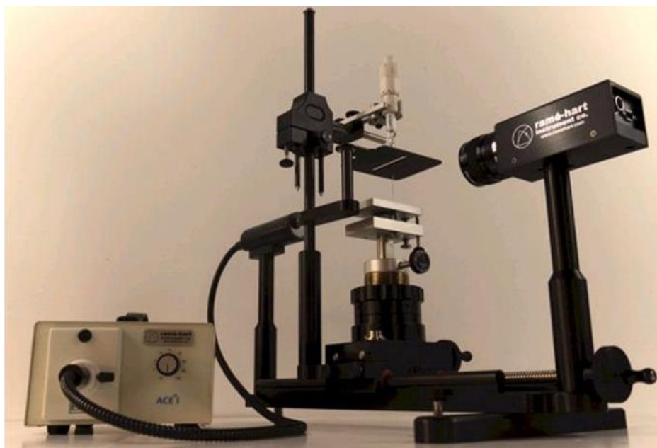
Figure 2.1.3 Image of Ramé-Hart goniometer (NJ, USA) equipment
