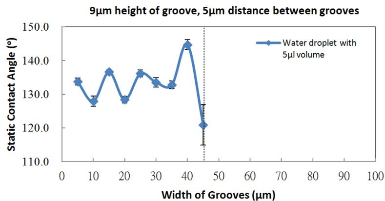
**Figure 3.12** Static contact angle as a function of geometric parameters of the micro patterns on PMMA surfaces with different groove width values with 5 $\mu$ l volume. A dotted line represents the boundary of wetting transition.
