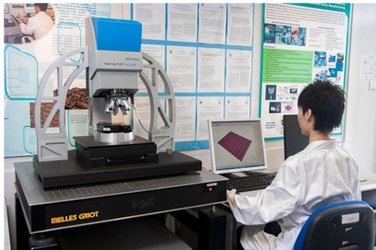
**Figure IV-1** Alicona IFM G4 3D Optical Surface Profiler.
