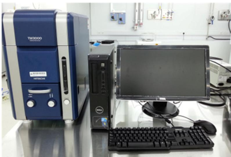
**Figure II-1** TM3000 Hitachi Electron Microscope.
