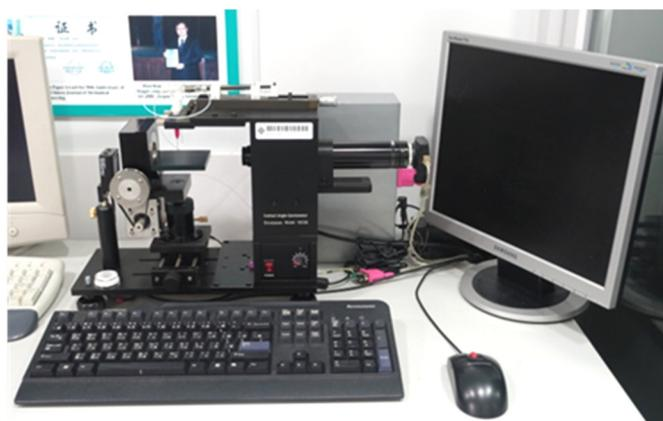
**Figure VI-1** Sindatek Model 100SB Video-based Optical Contact Angle Meter.
