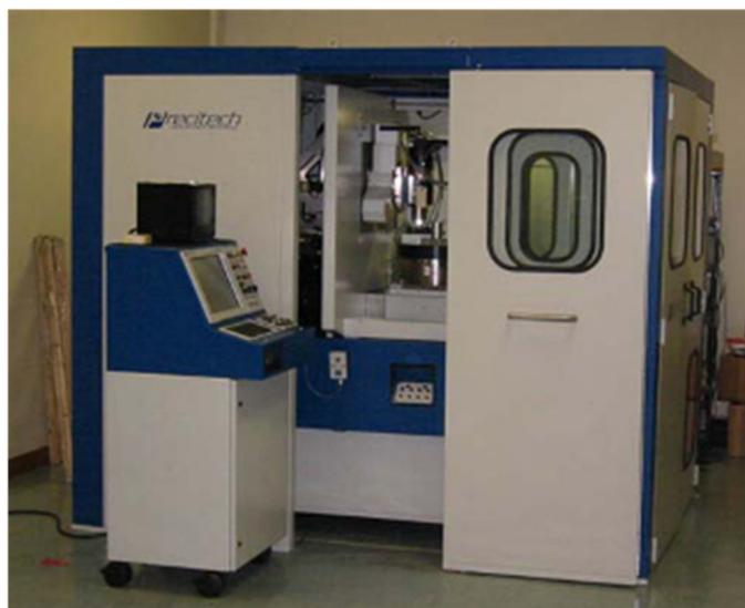
**Figure I-1** Precitech Freeform 705G Ultra-precision raster milling machine.
