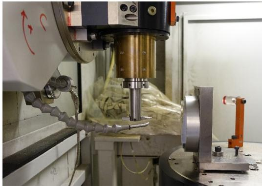
**Figure 2.11** Ultra-precision raster milling.
