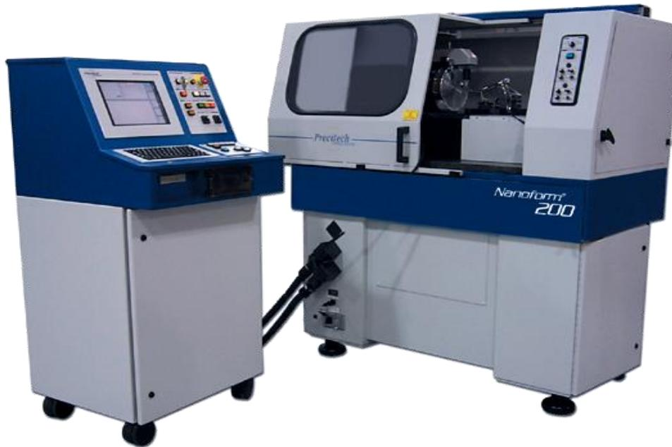
The Nanoform 200 is a two-axis computer controlled diamond turning machine. Its two linear axis are equipped with hydrostatic oil bearing while an aerostatic, slot-type thrust bearing is utilized for the spindle. The fast & slow tool servo, oil hydrostatic rotary B-axis and grinding spindle are optional. The key features of this machine are:
