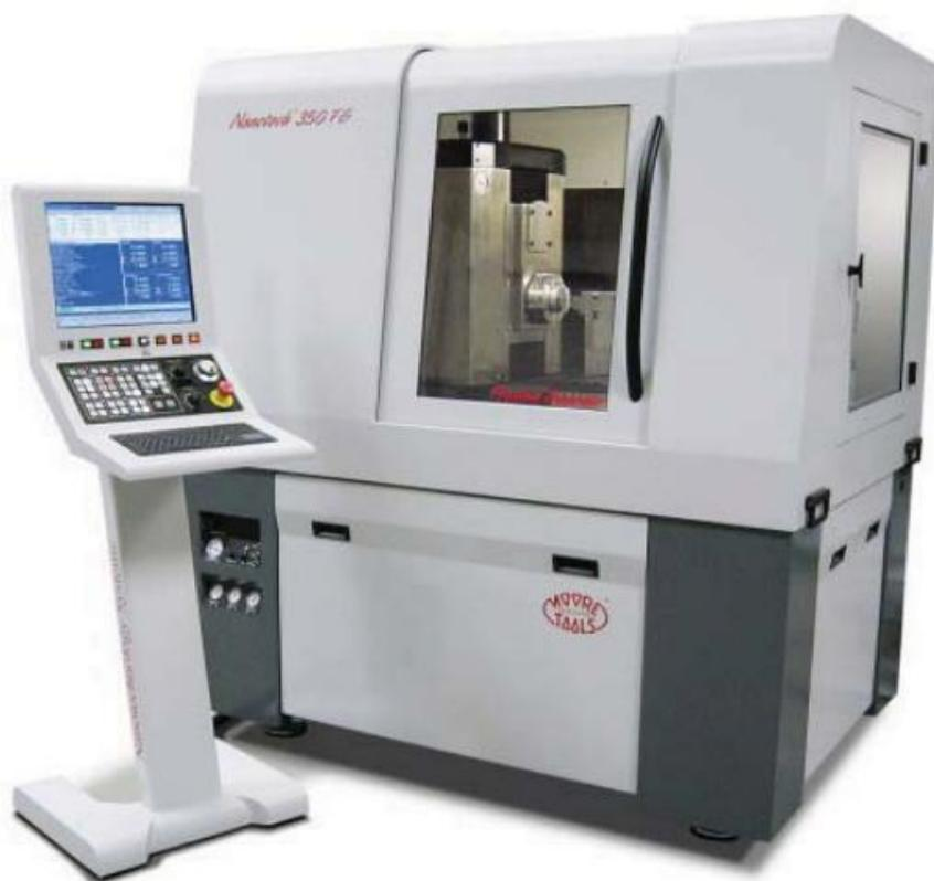
The Moor Nanotech 350FG is a 4-axis computer controlled ultra-precision machine. This ultra-precision machine is capable of machining a variety of surfaces including aspheric and toroidal axisymmetric surface, freeform surfaces machined with slow tool servo machining and raster flycutting. The key features are:
