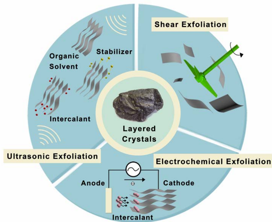
Figure 2.4. Schematic illustration of Liquid-based direct exfoliation of bulk-layered crystals.
