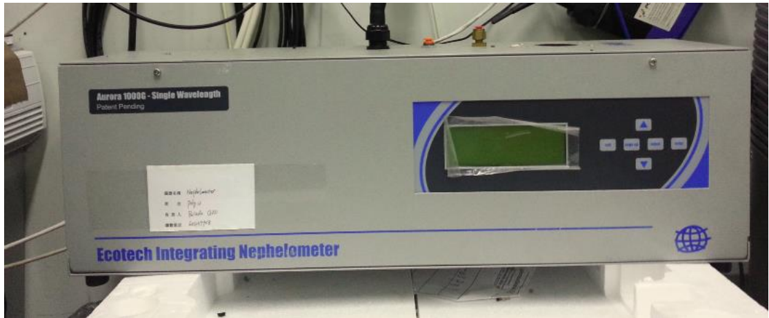
Photo 5. Nephelometer Ecotech M9003
