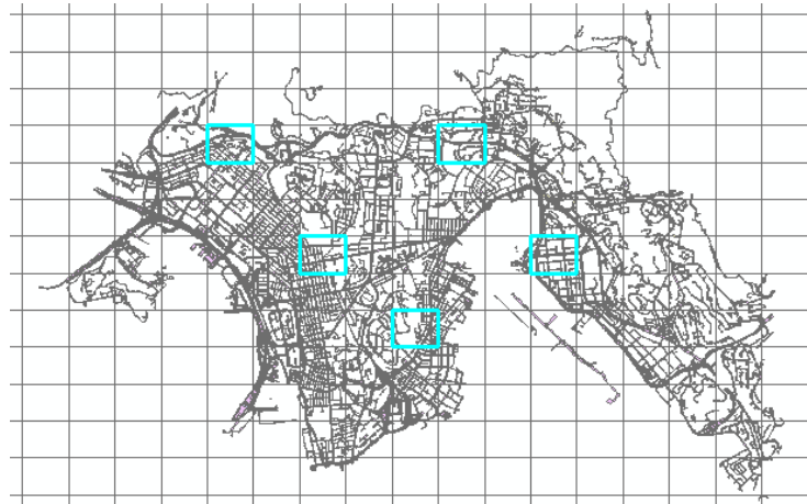
Figure 2.7 (a) Example of area-guided sampling using random selection
