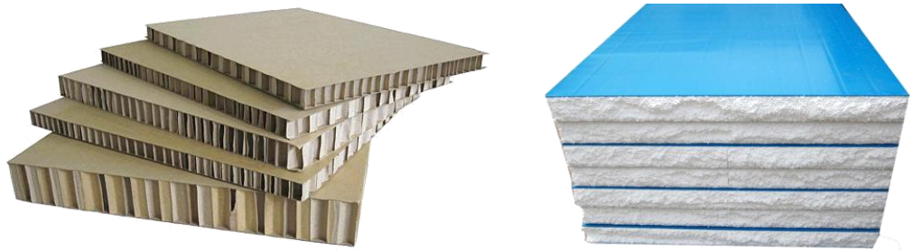
Figure 1.4 Two types of sandwich structure.
