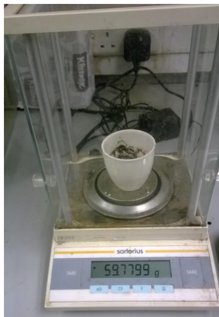
Figure 3. 16 Electronic scale for weighing samples with sensitivity of 0.1 mg, SARTORIUS, BL2105
