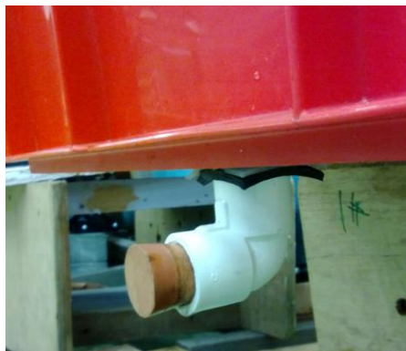
Figure 3. 32 Sealing for the drainage adapter
