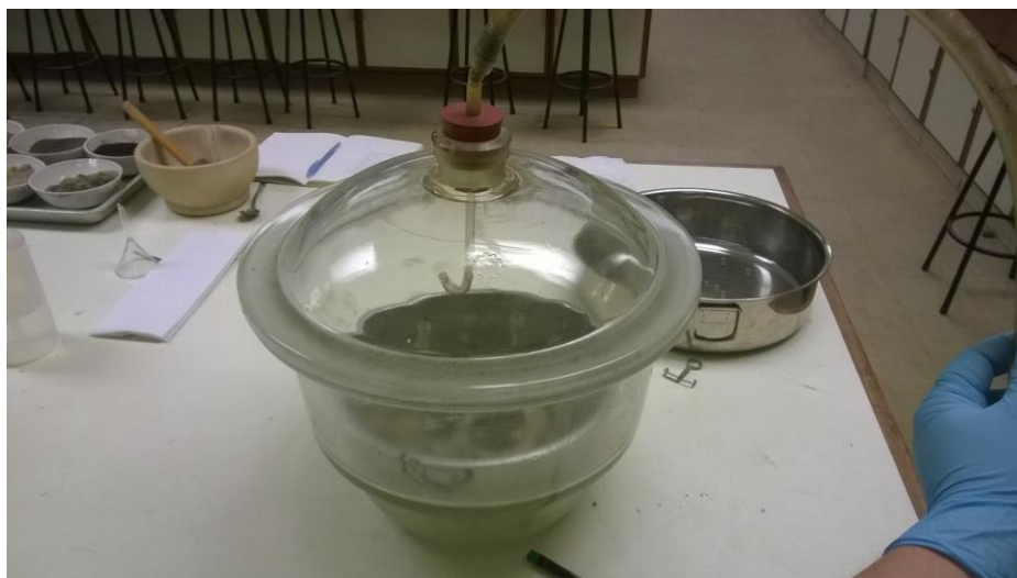
Figure 3. 66 Extraction of air bubbles in the substrates under vacuum pressure
