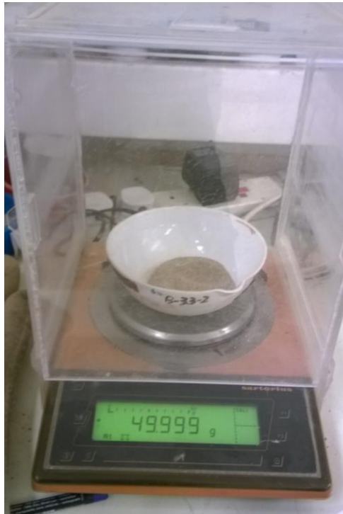
Figure 3. 63 Electronic scale for weighing the substrate specimen
