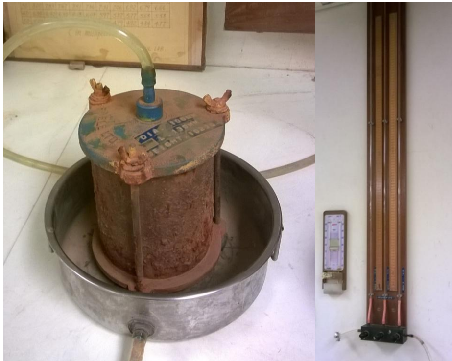
Figure 3. 67 Falling head permeability apparatus and the standpipes in the diameter of 1.5, 3.0 and 5.0 mm
