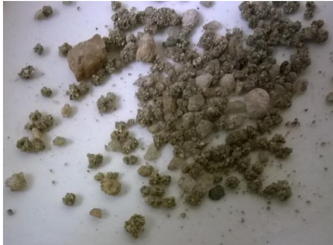
Figure 4. 10 Fine particles adhered by activated sludge to form large particles
