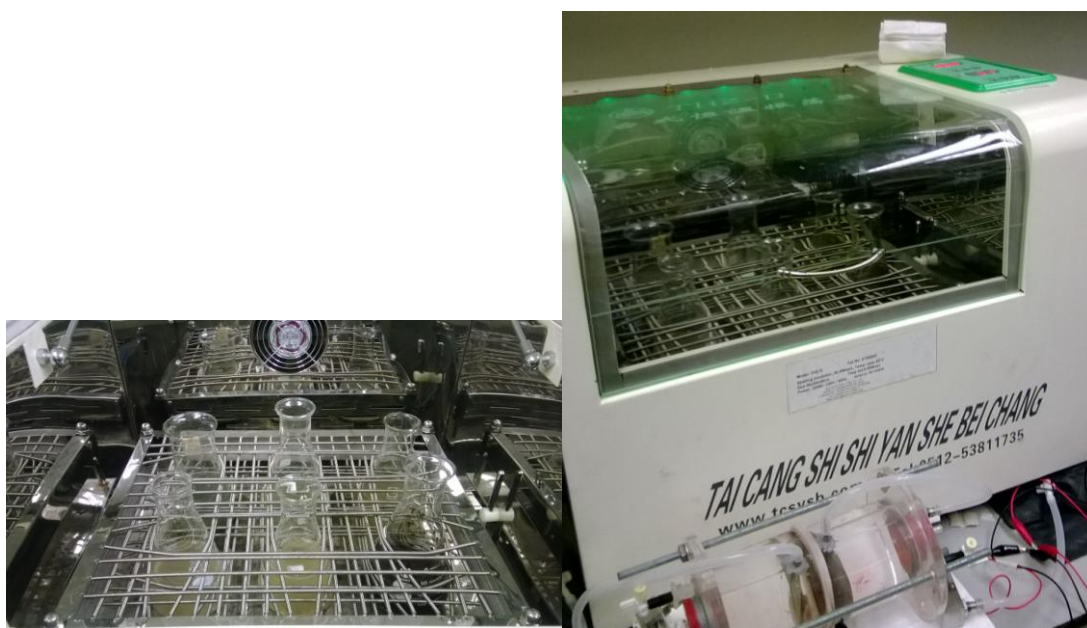
Figure 3. 54 Mixing of the samples in the shaking incubator (TAI CANG, Model: THZ-D, rpm 30~280) at the rpm of 120 for 1 hr
