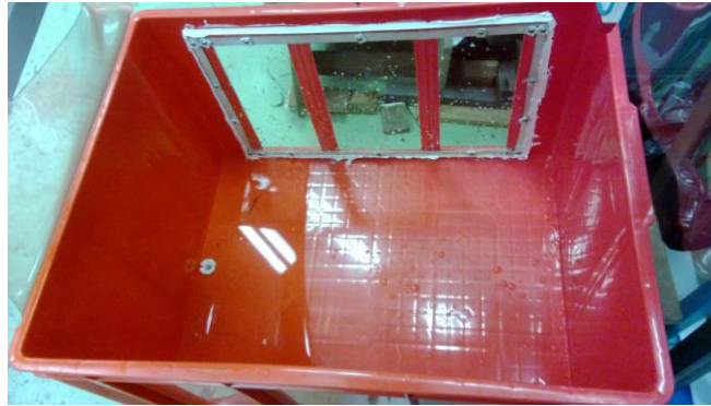
Figure 3. 31 Water sealing test on the experiment tank
