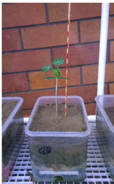
Figure 3. 62 Graduated stick inserted in each growing case
