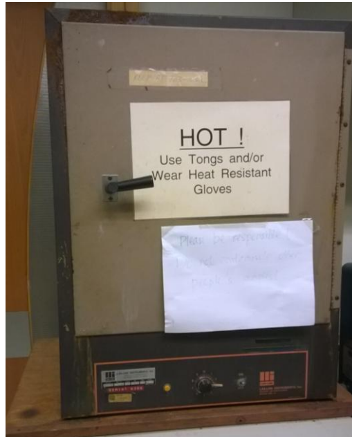
Figure 3. 15 Oven for drying at 105 \pm 1^\circ\text{C} , LAB-LINE INSTUMENTS, Inc. Cat NO.3524
