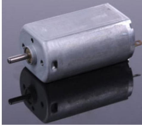
Figure 3. 38 Model ship motor (the axle is 2.1mm; operates within 1.0~9.0 V; 3833 RPM at 6V)
