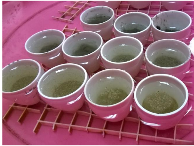
Figure 3. 23 Perforated Gooch crucibles contained samples and soaked in over surface distilled water basin
