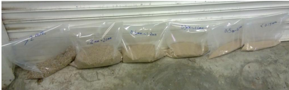
Figure 3. 13 Sieving of sand into different particle size groups
