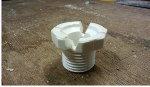
Figure 3. 30 Design of drainage adapter for experiment tank
