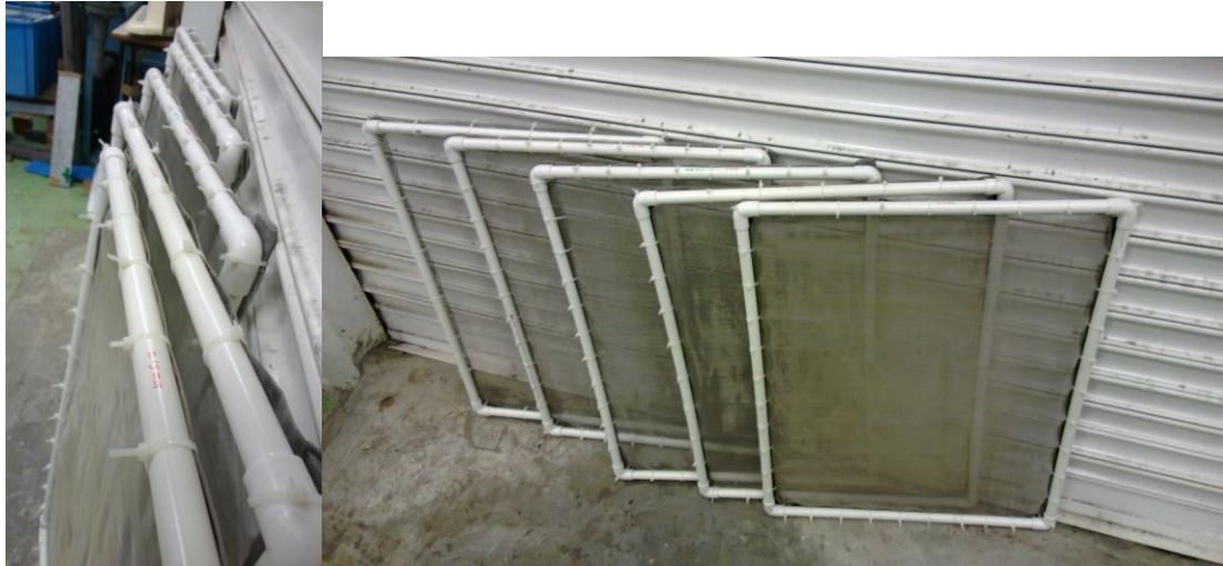
Figure 3. 12 Stainless steel sieves with pore size of 150, 300, 600, 1200 and 2000 \mu m
