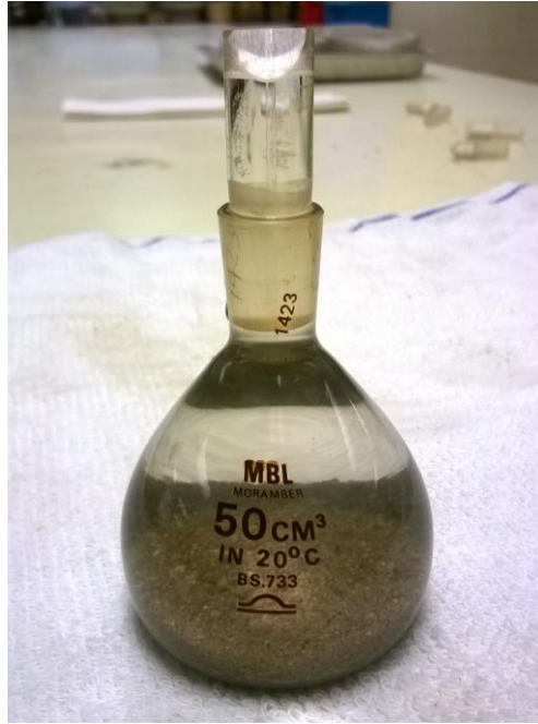
Figure 3.67 Pycnometers saturated by distilled water
