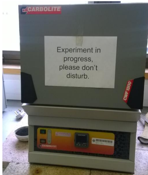
Figure 3. 17 Programmable furnace for ignition CARBOLITE, CWF 12/5
