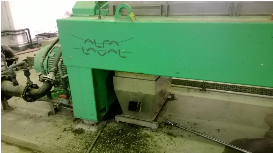
Figure 3. 10 Sludge sampling port on a centrifugal thickening facility
