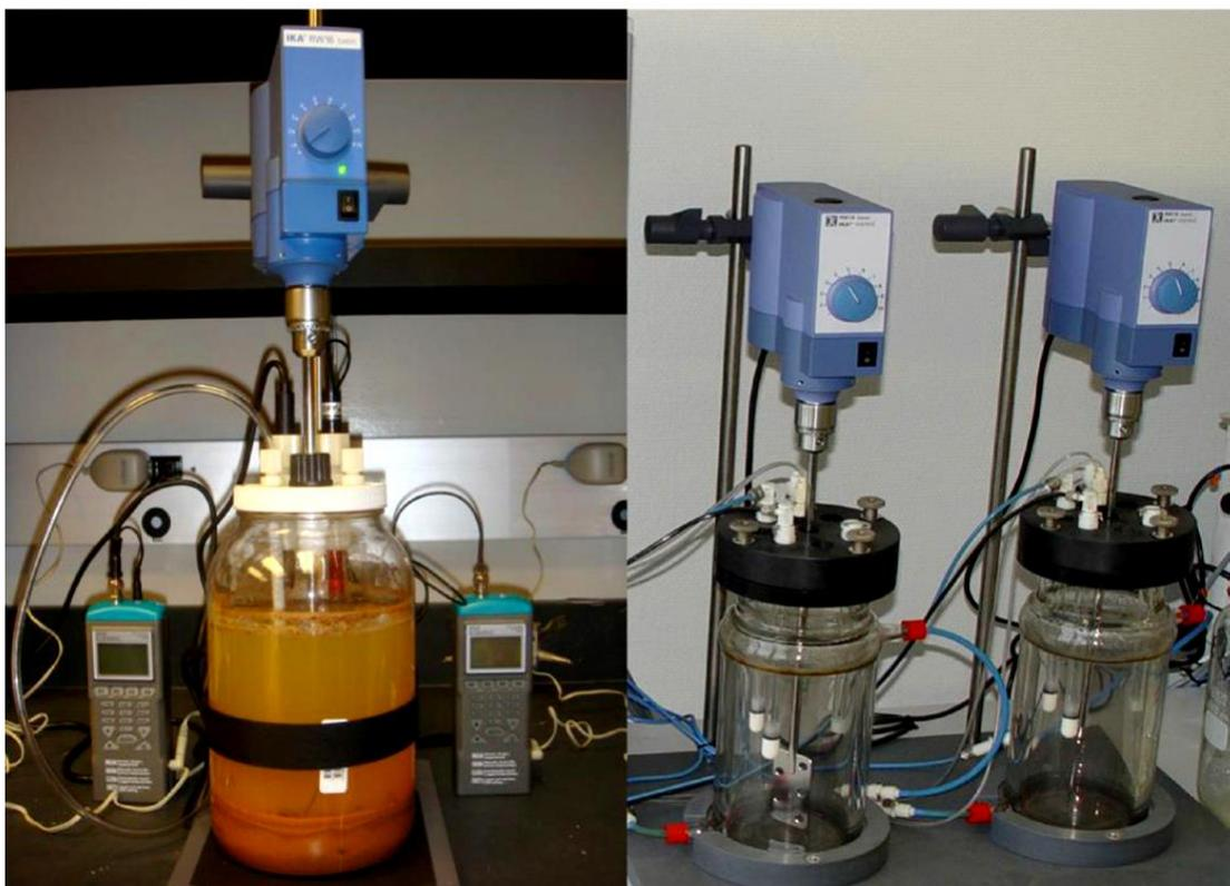
**FIGURE 3-2** A schematic of a soil microcosm (above), and photos of a microcosm with automatic  $E_H$  and pH measuring system (bottom left) and microcosms with temperature control system (bottom right) (Yu and Rinklebe, 2011).
