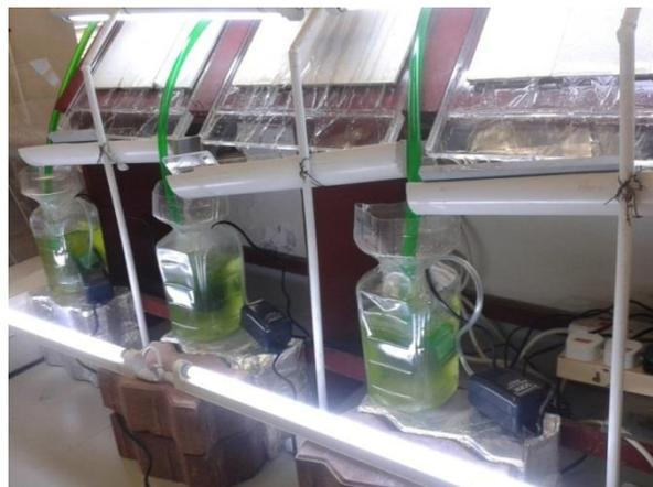
Figure 3.7 Accelerated algae fouling test set-up
