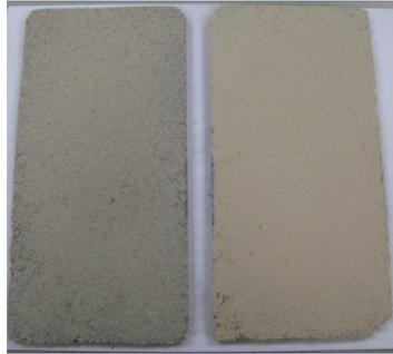
Figure 3.13 Left, 10 g and right, 37 g of dust were accumulated per  $\text{m}^2$  of surface
