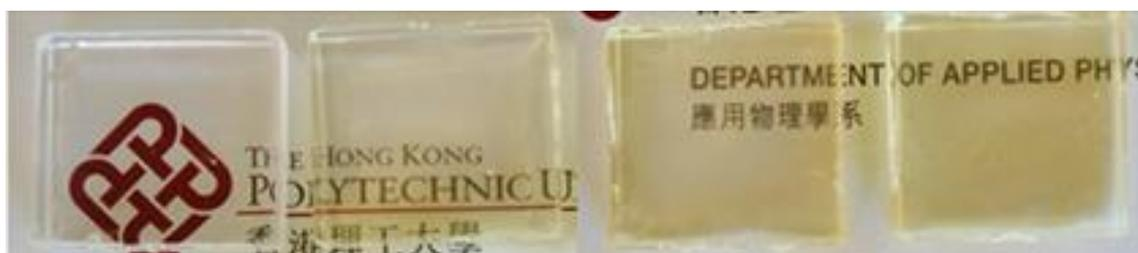
Fig. 5.10 Digital photographs of prepared WS<sub>2</sub>/PMMA composites, they are S500, S1000, S5000 and S7000 from the left to right, respectively.
