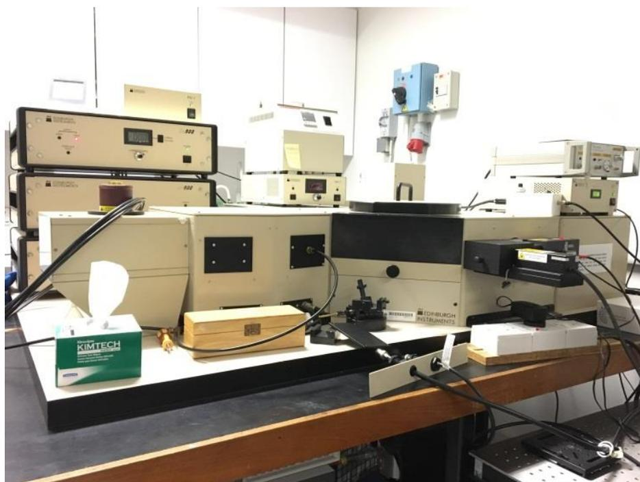
Fig. 2.4 Digital image of the photoluminescence spectrophotometer.
