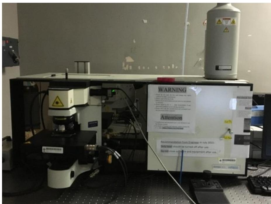
Fig. 2.5 Digital image of the Raman spectrophotometer.
