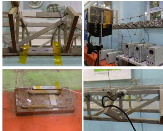
Figure 9.1 Sensor installations in the test: FBG sensor (top left), installed FBG sensors for temperature compensation (bottom left), laser displacement transducers (top right), and accelerometers (bottom right).
