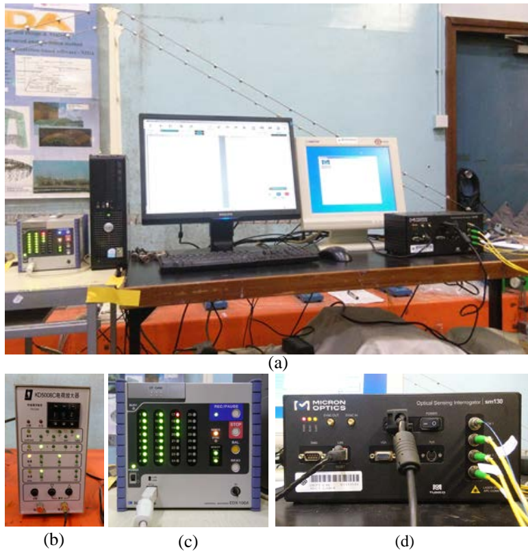
Figure 9.4 Data acquisition systems in the test: (a) the overall view of the system, (b) KD 5006 charge amplifiers, (c) KYOWA EDX-100A data acquirer and (d) optical sensing interrogator sm130.
