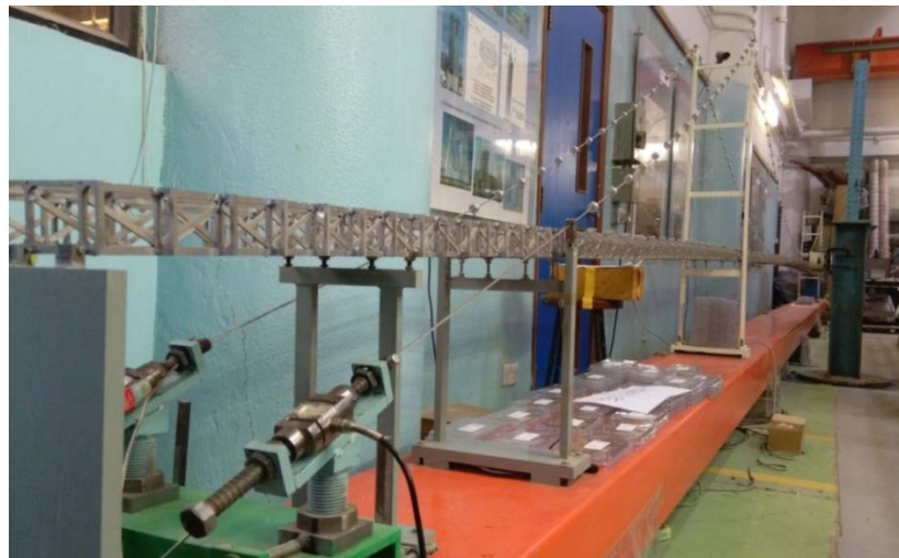
Figure 8.2 Tsing Ma Bridge testbed in the laboratory
