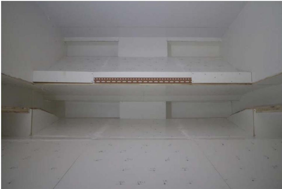
**Figure 3-5 The balcony in the scale model in case 1 and case 2**
