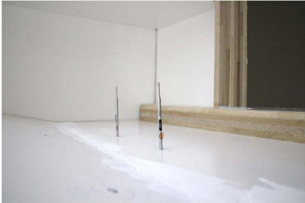
**Figure 3-11 1/8 inch microphones at measurement position**
