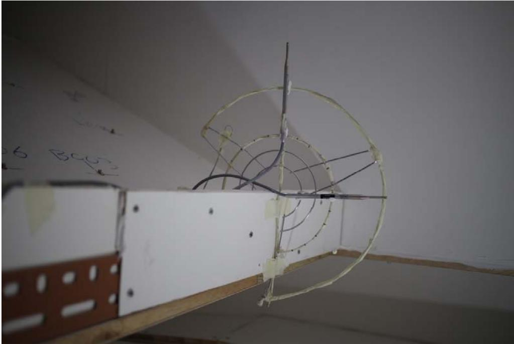
**Figure 3-10** Microphones mounted on the tailor-made measurement rack at one of the balcony edge positions
