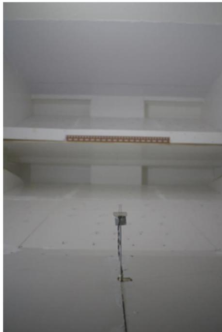
**Figure 3-8 Spark source mounted at the source position.**
