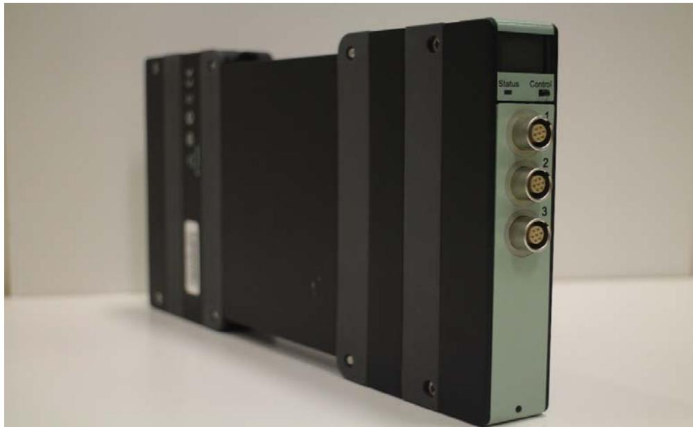
**Figure 3-12 High frequency LAN-XI data acquisition hardware, Pulse system used in scale model measurement**
