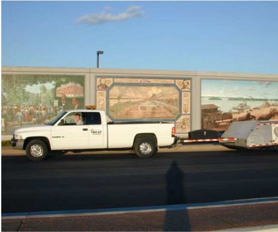
Figure 2.5. Typical CPX trailer measurement (Source from Bernhard et al., 2005)
