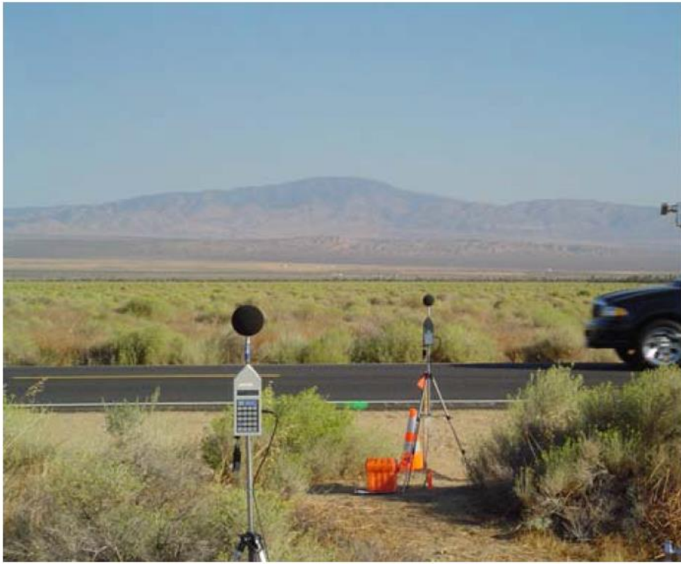
Figure 2.3. Typical measurement setup for SPB. (Source from Bernhard et al., 2005)
