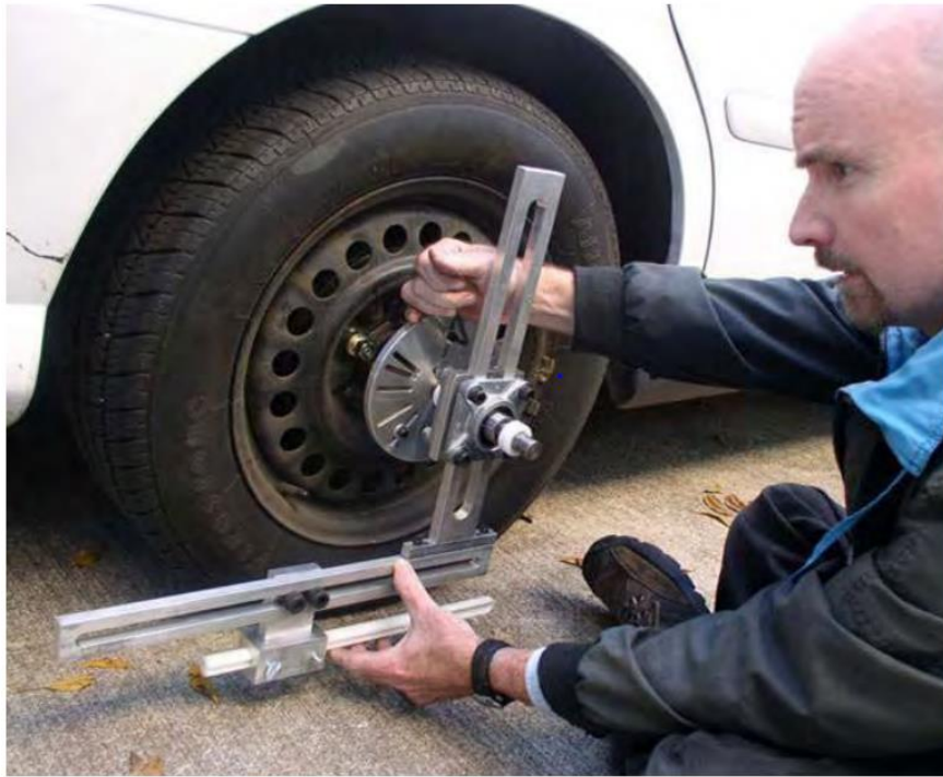
Figure 2.4. OBSI jig being attached to wheel hub on test vehicle (Source from Trevino and Dossey, 2006)
