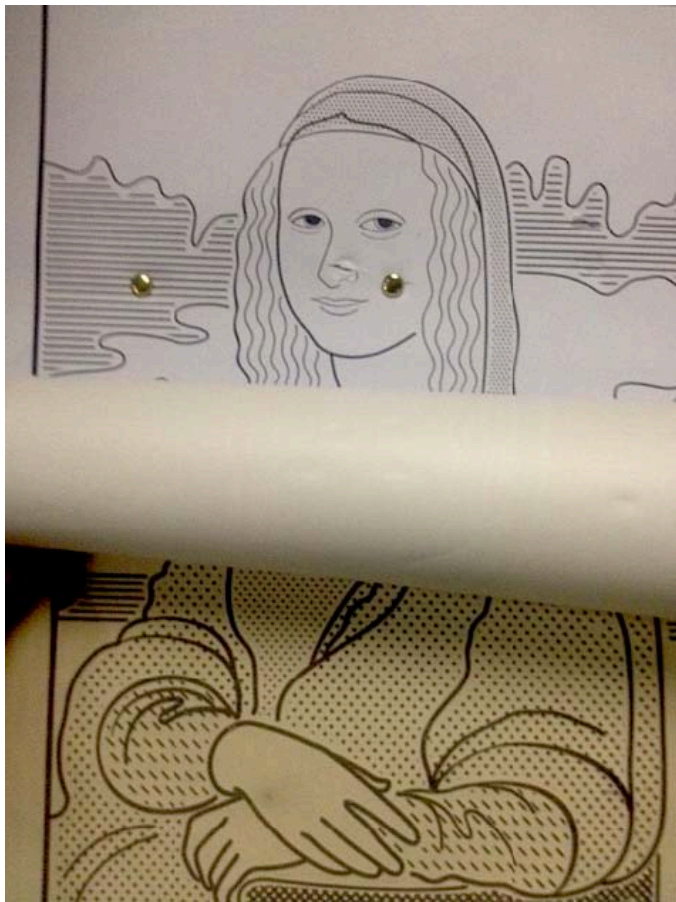
Figure 13: HAID simulated tactile paper prototype – To create the sensation of pressing a button to activate the ‘point description’ function on the prototype, metal pins were embedded in the back of the diagram. The diagram was glued to a form-board, which stimulated haptic force feedback when participants pressed on the tactile surface.
