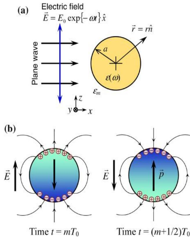
Figure 2.7 Schematic description of the optical response of a particle in the spherical shape. (a) Graph of a homogeneous nanosphere under the illumination of a plane incident light; (b) the homogeneous nanosphere is polarized by the external electric field and the oscillating dipole enhances the local electric field and radiates energy in turn. The scattering is ignored.<sup>48</sup>
