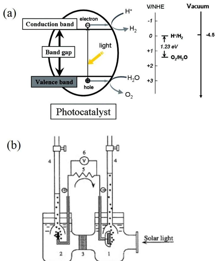
Figure 2.1 (a) Schematic representation of a photoelectrochemical cell.<sup>20,22</sup> (b)
