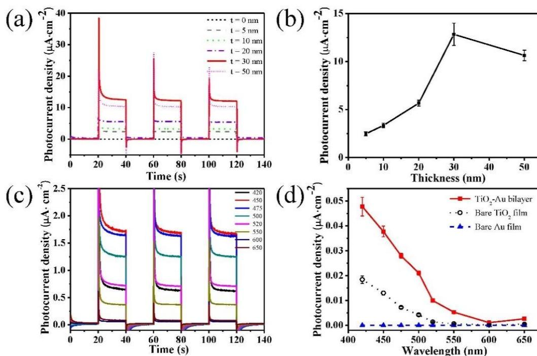
Figure 4.10 (a) *I-t* plots and (b) photocurrent intensities of the TiO<sub>2</sub>-Au bilayer samples with different TiO<sub>2</sub> thicknesses of 0, 5, 10, 20, 30 and 50 nm.; (c) *I-t* plots under the irradiation of monochromatic light; and (d) action spectra (i.e., photocurrent versus light wavelength) of the TiO<sub>2</sub>-Au bilayer with 30-nm-thick TiO<sub>2</sub> film (red line), the 30-nm-thick bare TiO<sub>2</sub> film (black line) and the bare Au film (blue line).
