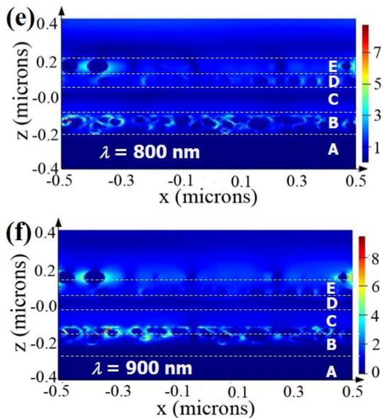
Figure 5.9 Distributions of electric field intensity for the perfect structure in the  $xz$  plane at six selected wavelengths: (a) 410 nm, (b) 500 nm, (c) 600 nm, (d) 700 nm, (e) 800 nm, and (f) 900 nm. The rough Au layer (i.e., Layer B) has always strong plasmonic resonance at different wavelengths and becomes the dominant absorber when the wavelength is longer than the plasmonic resonance wavelength 600 nm.
