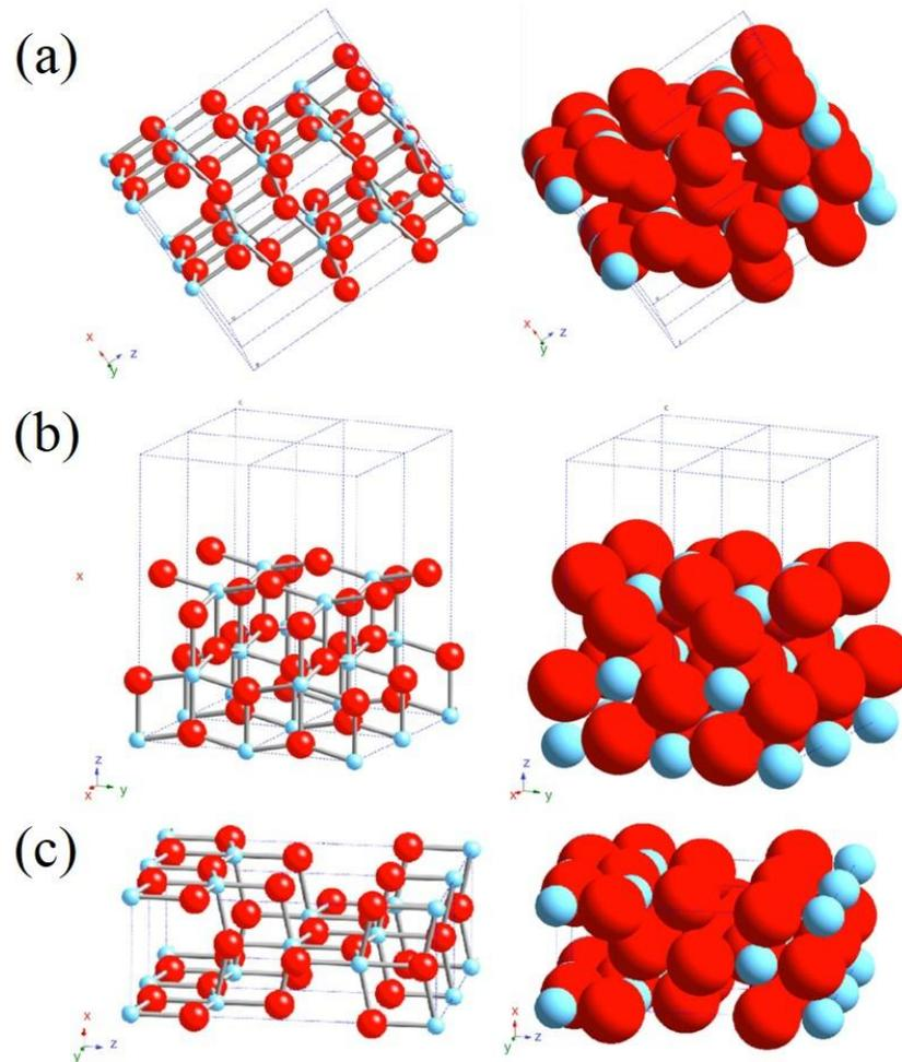
Figure 2.5 Schematic diagrams of three most prevalent anatase crystals with low-index faces: (a) (101); (b) (100); and (c) (001).<sup>95</sup>
