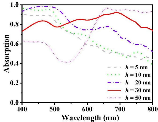
Figure 4.11 Simulated results of the absorption spectra of the TiO<sub>2</sub>-Au bilayer samples.
