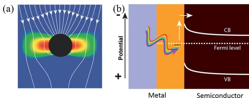
Figure 2.13 (a) The illustration of the energy flux (Poynting vectors) and the electric field intensity for an incident electromagnetic wave with an electric field in the plane of image; (b) hot electron injection from a metal into an n-type semiconductor.<sup>108</sup>
