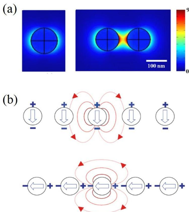
Figure 2.8 (a) Comparison of the electric field distributions between a single Au nanoparticle and nanoparticle dimer. (b) Schematic of the transverse and longitudinal resonant modes for near-field dipolar coupling of NPs.<sup>48</sup>
