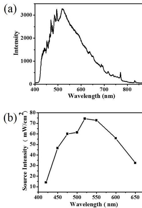
Figure 4.4 (a) Calibrated emission spectrum of the light source after the UV-cutoff filter (> 400 nm), the overall intensity is  $\sim 300 \text{ mW/cm}^2$  at the photoelectrode surface. (b) Calibrated optical intensities of the light source at different wavelengths when the narrow-band optical filters are used to get monochromatic light for the measurement of action spectrum.
