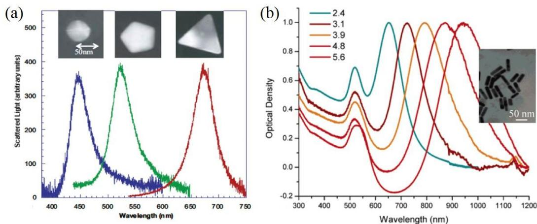
Figure 2.9 (a) Scattering spectra of single silver NPs with various shapes.<sup>104</sup> (b) Absorption spectra of Au nanorod with changed aspect ratios. Every curve appears two separate peaks corresponding to the transverse and longitudinal resonances.<sup>105</sup>
