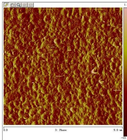
Figure 5.5 AFM surface profile of the rough Au layer under the TiO<sub>2</sub> layer. The area is 5  $\mu\text{m} \times 5 \mu\text{m}$ . The root mean squared (RMS) roughness is 11.0 nm.
