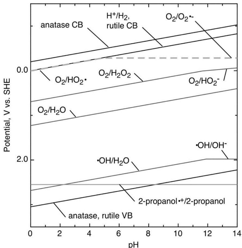
Figure 2.6 Energy bands of  $\text{TiO}_2$  as a function of pH.<sup>95</sup>
