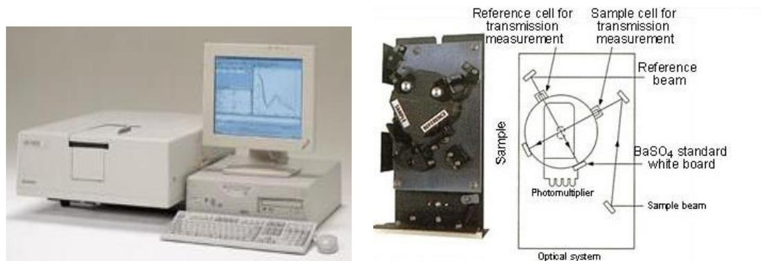
Figure 3.4 (a) Photograph of the UV-Vis spectrophotometer equipment and (b) the attachment ISR-240A integrating sphere.
