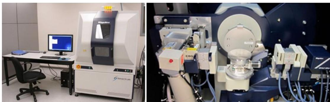
Figure 3.5 Digital image of the Smartlab X-ray diffractometer.
