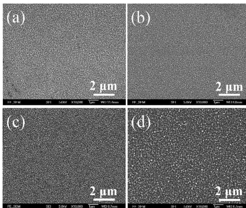
Figure 4.7 SEM surface morphologies of different layers in large area. (a) FTO glass; (b) Au NPs on the FTO glass, deposited by the sputtering process; (c) rough Au film on the FTO glass; (d) TiO<sub>2</sub> film deposited by the ALD method.
