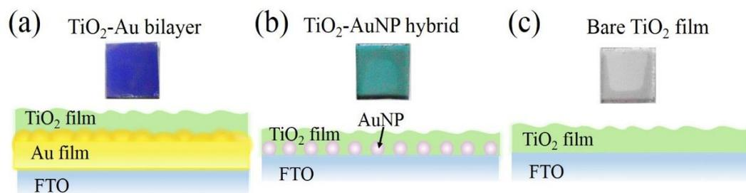
Figure 4.1 Photographs and schematic diagrams of the three samples, from left to right, (a) the TiO<sub>2</sub>-Au bilayer, (b) the TiO<sub>2</sub>-AuNP hybrid and (c) the bare TiO<sub>2</sub> film, each sample has the footprint of 1 cm × 1 cm.
