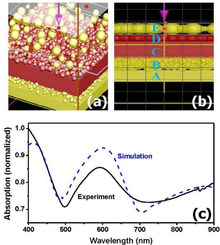
Figure 5.8 FDTD simulation. (a) Perspective view of the representative structure of black absorber for simulation. (b) Cross-sectional view in the  $xz$  plane. (c) Simulated absorption spectrum (blue dashed line) matches approximately the experimentally measured spectrum (black line).
