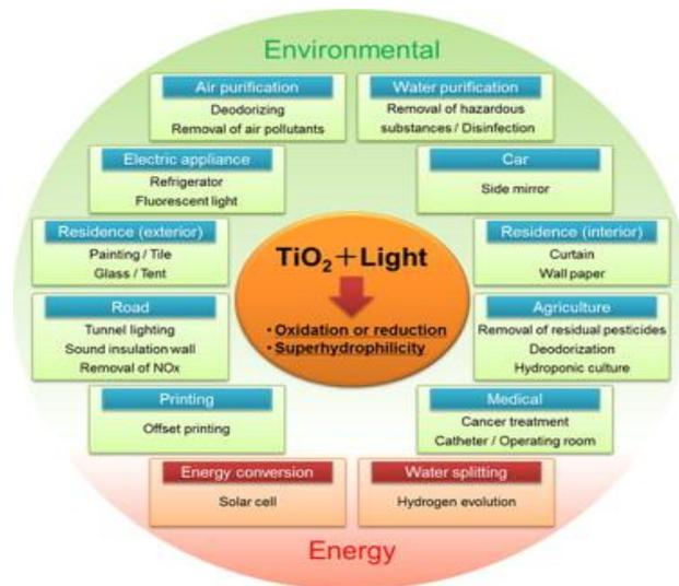
Figure 1.3 Application of  $\text{TiO}_2$  photocatalysis.<sup>26</sup>
