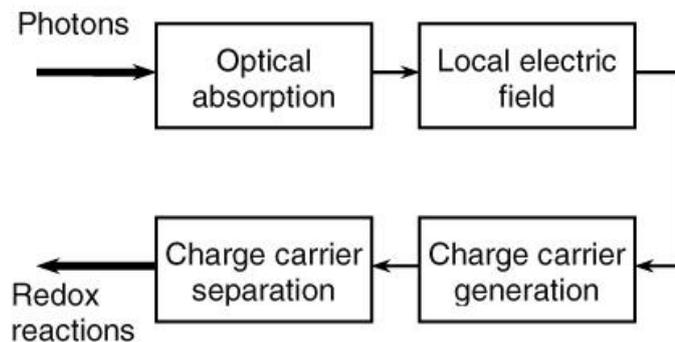
Figure 2.11 Plasmonic enhancements for the primary steps of photocatalysis.<sup>48</sup>
