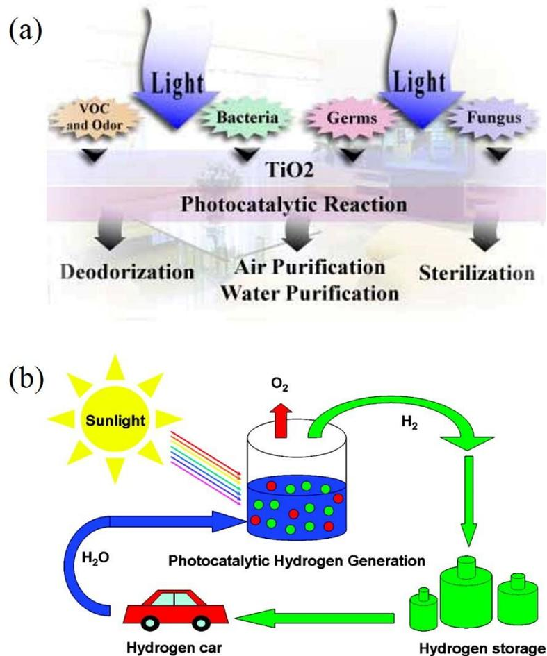
Figure 1.2 Schematic diagram of (a) photocatalytic degradation (from <http://gamma-nano.ca/what-is-a-photocatalyst/>) and (b) photocatalytic hydrogen generation application.<sup>22</sup>
