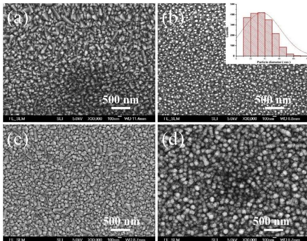
Figure 4.6 Scanning electron micrographs of the surface morphologies of different layers in the samples. (a) FTO glass; (b) Au NPs on FTO glass, deposited by the sputtering process; (c) rough Au film on FTO glass; (d) ALD-deposited TiO<sub>2</sub> film on the rough Au film. The inset in (b) is the histogram of the size of Au NPs.
