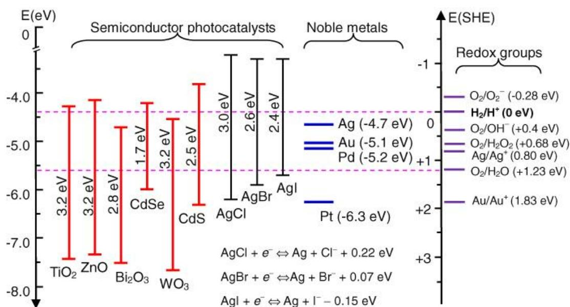
Figure 2.2 Energy band position of several popular photocatalysts, including the valence and conductive bands of the semiconductor, the work functions of the noble metals and the electrochemical potentials of the redox groups.<sup>48</sup>
