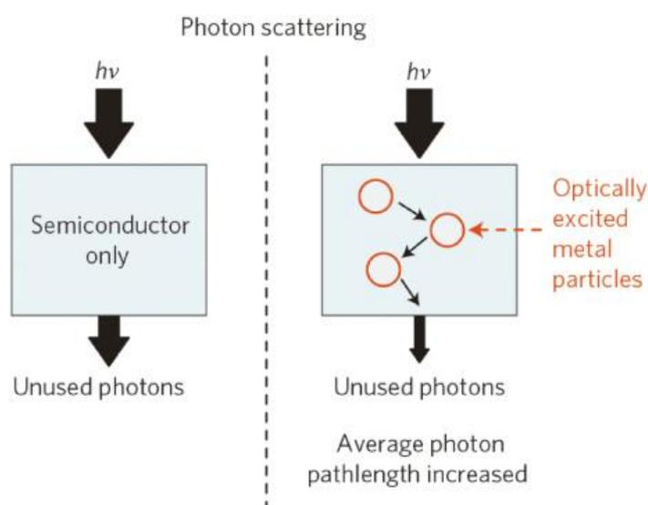
Figure 2.12 Scattering effect of the metal NPs leads to an absorption enhancement through increasing the average photon path length in the metal/semiconductor composite.
