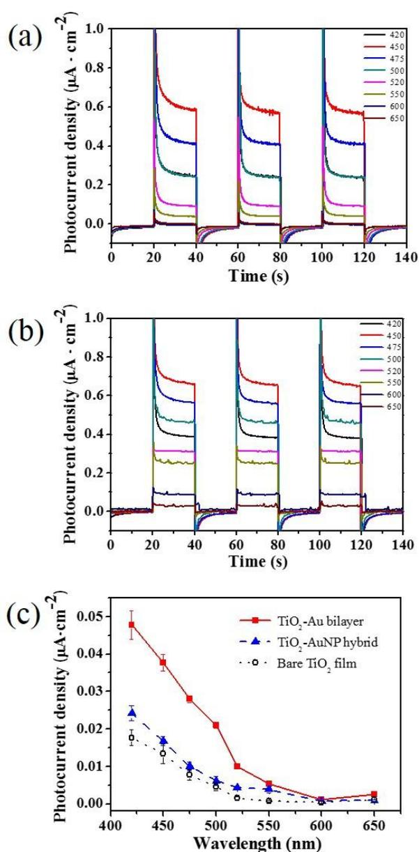
Figure 4.5  $I-t$  plots of (a) the bare  $\text{TiO}_2$  film and (b) the  $\text{TiO}_2$ -AuNP hybrid under monochromatic lights of 420, 450, 475, 500, 520, 550, 600 and 650 nm, respectively. (c) Action spectra (i.e., photocurrent versus light wavelength) of the  $\text{TiO}_2$ -Au bilayer (red solid line), the  $\text{TiO}_2$ -AuNP hybrid (blue dashed line) and the bare  $\text{TiO}_2$  film (black dotted line). In these three samples, the  $\text{TiO}_2$  layers are all 30 nm thick.
