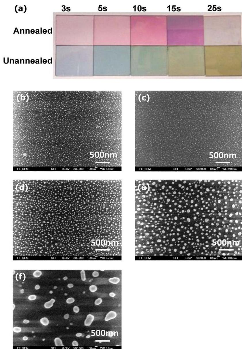
Figure 3.3 (a) Photographs of the Au films with the sputtering time of 3 s, 5 s, 10 s, 15 s and 25 s, before and after annealing at 500 °C; SEM images of the Au nanoparticles after annealing the Au films with the sputtering time of (b) 3 s; (c) 5 s; (d) 10 s; (e) 15s and (f) 25 s. Before annealing, the colors of the Au films are deep. After annealing, the films turn to lighter color and are mostly pink. For the sizes of Au nanoparticles, they increase with longer deposition time.
