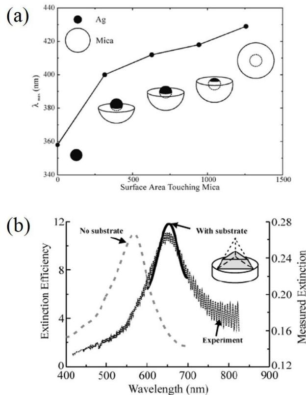
Figure 2.10 (a) the resonant wavelength shifts with the embedment state of the silver nanosphere (radius 10 nm) into the mica shell. (b) Comparison between the discrete dipole approximation (DDA) and experimental results for the effect on the extinction of a truncated tetrahedron.<sup>88</sup>
