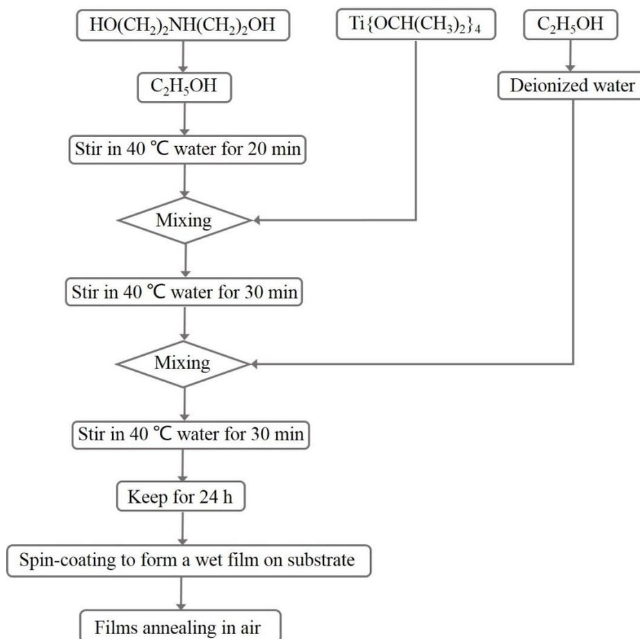
Figure 3.1 Scheme of the overall synthesis process developed to TiO<sub>2</sub> sol-gel thin films.
