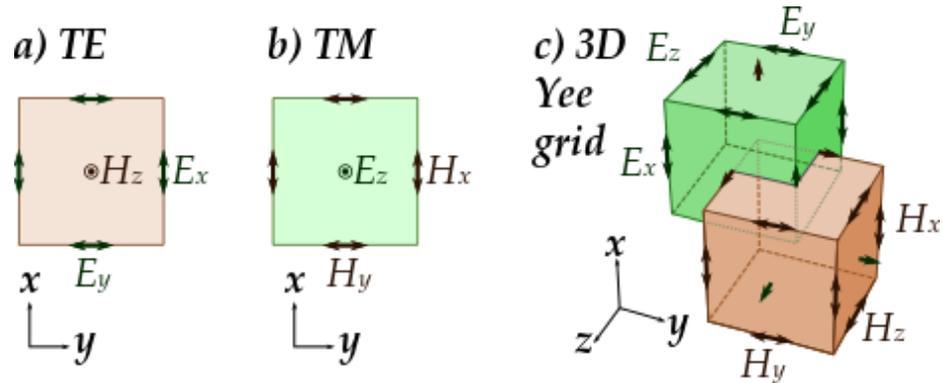
Figure 3.6 Illustration of a standard Cartesian Yee cell used FDTD, which electric and magnetic field vector components are distributed, from Wikipedia.
