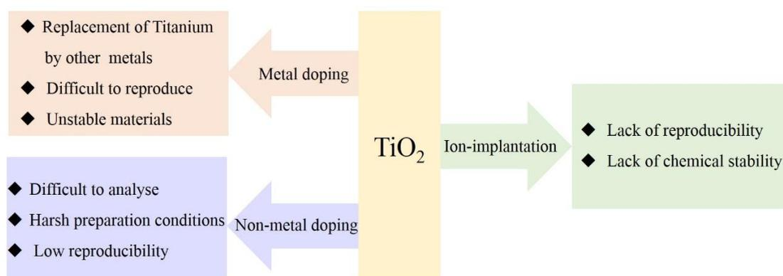
Figure 2.3 Pros and cons of the two alternative doping methods used to achieve visible-light photoresponse in  $\text{TiO}_2$ .
