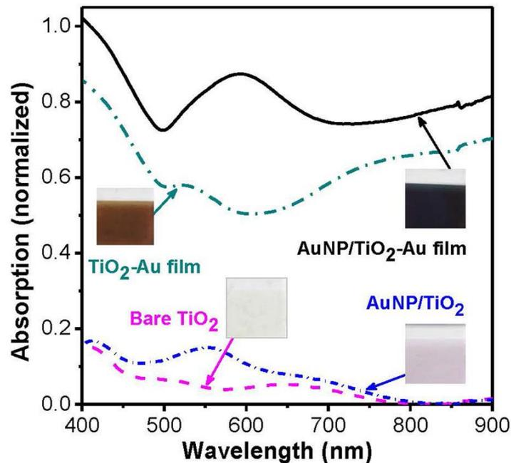
Figure 5.6 The measured absorption spectra of different film samples. The insets show the photos of the films. The bare TiO<sub>2</sub> film presents very low absorption, the AuNP/TiO<sub>2</sub> film has also low absorption but a plasmonic absorption peak at ~560 nm, the TiO<sub>2</sub>-Au film shows a much enhanced absorption, where the AuNP/TiO<sub>2</sub>-Au film exhibits strong absorption (> 72%) over the whole range of 400 – 900 nm and the maximum absorption of 91% at ~600 nm.
