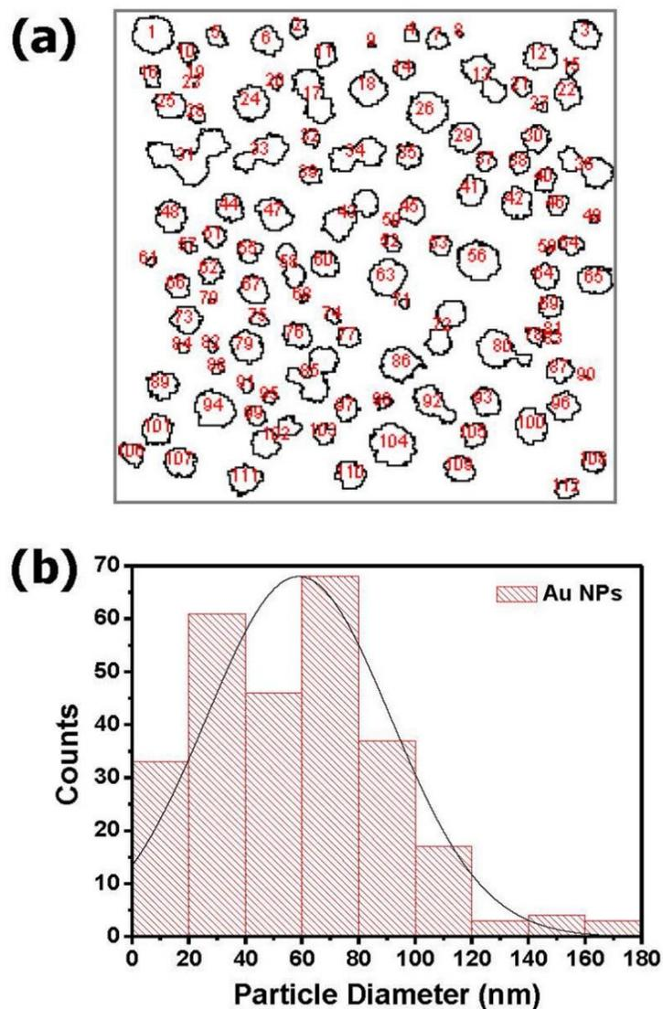
Figure 5.2 (a) Profile of Au nanoparticles in a small region of Figure 5.1(d). (b) Histogram of the size of Au nanoparticles in Figure 5.1(d), as analyzed by using the free software tool ImageJ.
