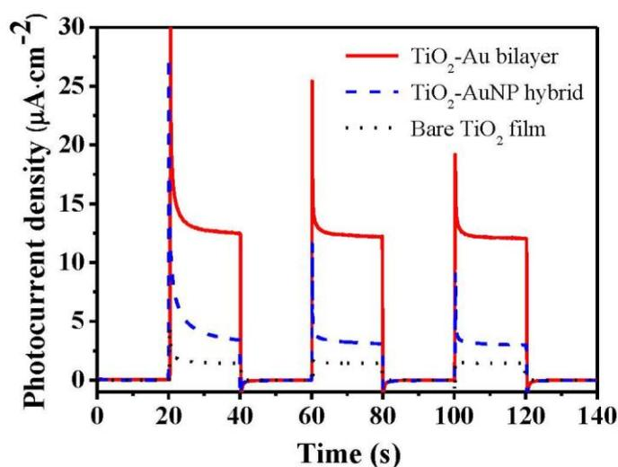
Figure 4.3 The absorption spectra and (b) *I-t* plots of the TiO<sub>2</sub>-Au bilayer (red solid lines), the TiO<sub>2</sub>-AuNP hybrid (blue dashed lines) and the bare TiO<sub>2</sub> film (black dotted lines), respectively. The TiO<sub>2</sub> films of the three samples are all 30 nm thick. The potential for the *I-t* measurement is 0 V vs SCE (saturated calomel electrode).
