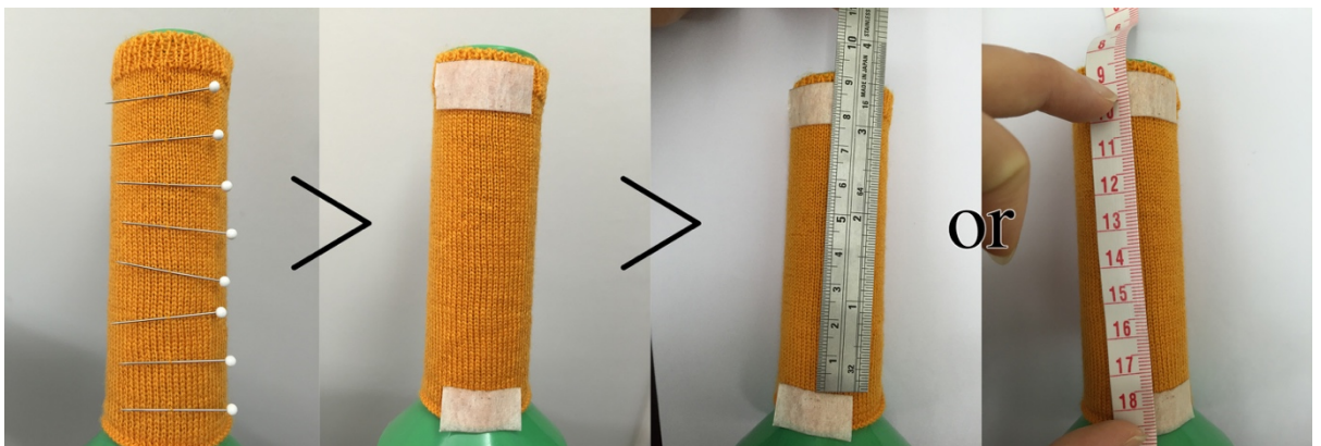
Figure 4.13 The procedures of measuring cpc with counting 70 successive loops
