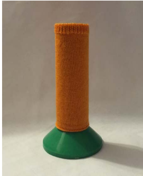
Figure 4.10 An image of the finished 3D knitted shape of zero Gaussian curvature on the target object
