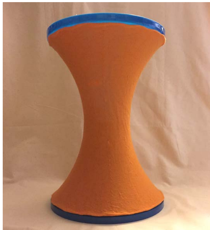
Figure 6.8 The knitted shape of surface with negative Gaussian curvature on the target
