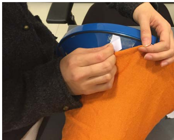
Figure 6.9 Applying double tape to the target edge to hold the fabric edge
