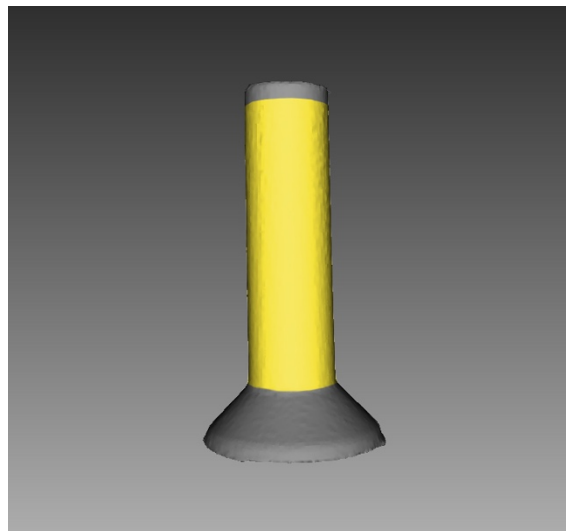
Figure 4.1 A digital image of the shape with a surface with zero Gaussian curvature indicated in yellow
