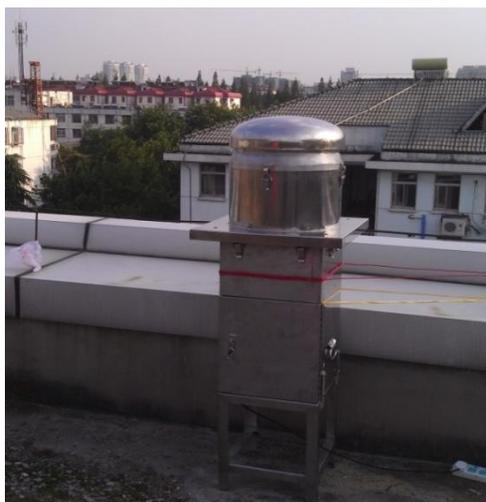
Figure 3-5 The high-volume PM<sub>2.5</sub> sampler.
