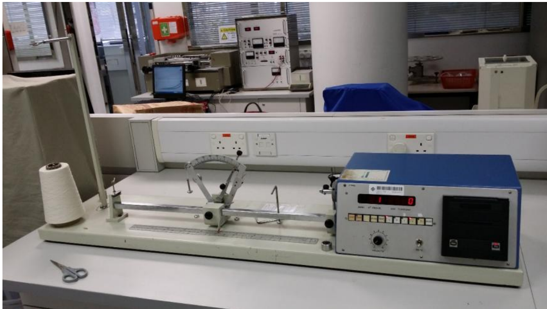
Figure 4.10 Mesdan electronic yarn twist tester (Author, 2017)
