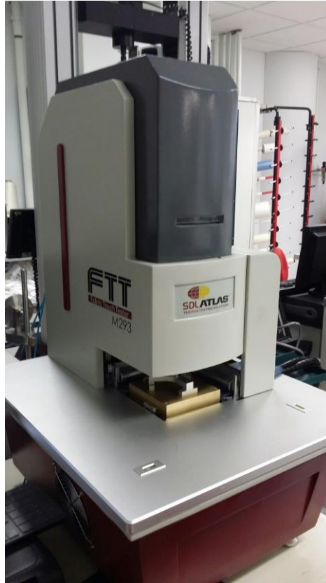
Figure 4.16 SDL ATLAS Fabric Touch Tester M293 (Author, 2017)
