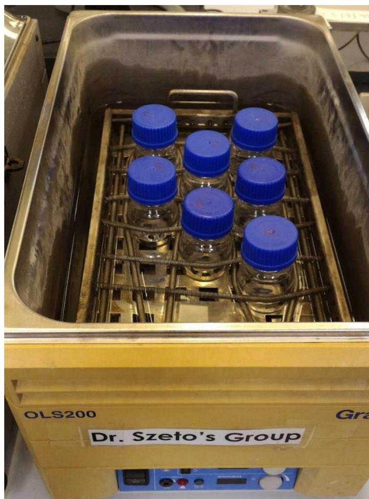
Figure 3.3 Biosorption experiments conducted in OLS 200 orbital shaking water bath (Grant Instruments).
