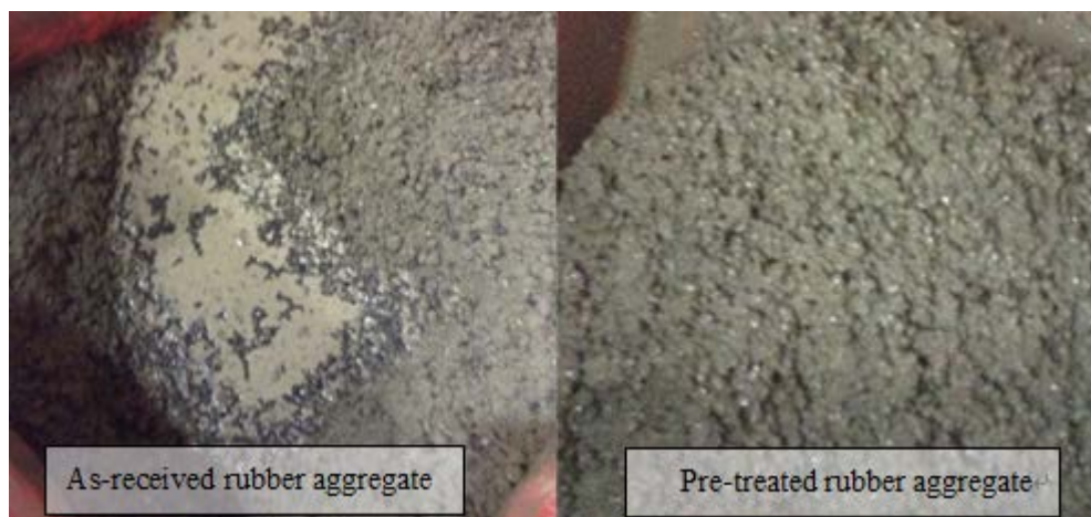
Figure 4-33 Improved workability when surface modification applied to rubber aggregate
