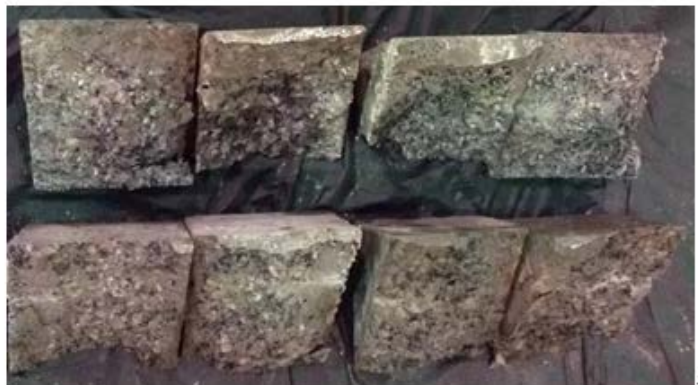
(b) As-received rubberized concrete-matrix bonding failure
