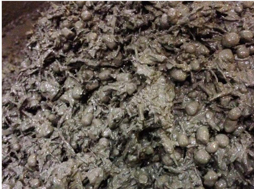
Figure 4-32 Inconsistency of fresh mixed rubberised concrete with high volume recycled rubber aggregate incorporation
