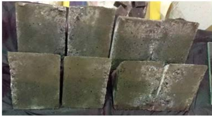
(a) Pre-treated rubberized concrete-matrix bonding failure
