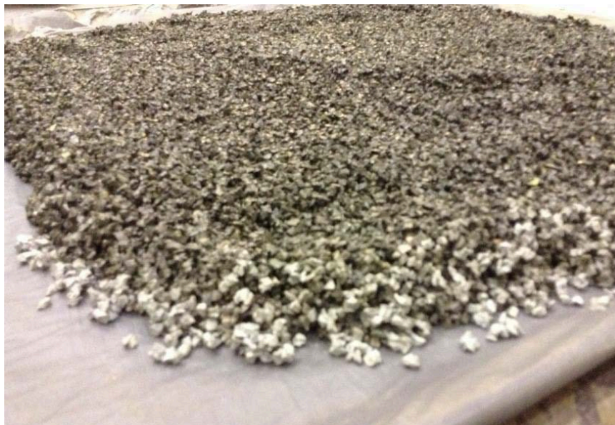
Figure 3-2 Applying the coating method on the surface of recycled rubber aggregate
