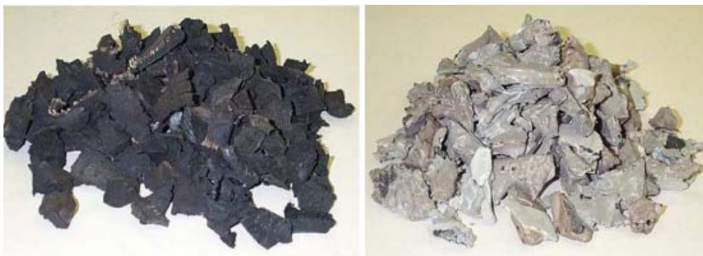
Figure 2-9 Recycled rubber aggregate before and after coating (Pacheco-Torgal et al. 2012)
