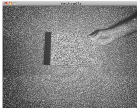
Figure 2.3 An image of normally invisible grid of dots from infrared projector
