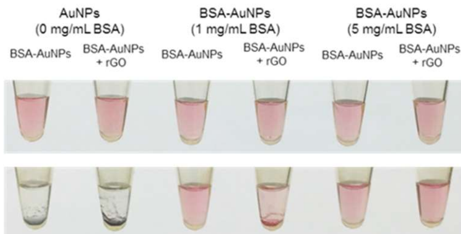
Figure 3.16. Photograph showing the effect of different BSA concentrations (0, 1, and 5 mg mL -1 ; concentration of AuNPs was fixed at 20 nM) in the preparation of BSA-AuNPs on the co-precipitation of BSA-AuNPs with rGO. The concentrations of BSA-AuNPs and rGO were 2 nM and 8.75 µg mL -1 , respectively. The incubation of rGO in aggregation buffer was conducted at room temperature for 1 h, followed by the addition of BSA-AuNPs. The photograph was taken before (top) and after (bottom) the 1 h incubation at 65 °C. Samples without rGO were included for comparison.
