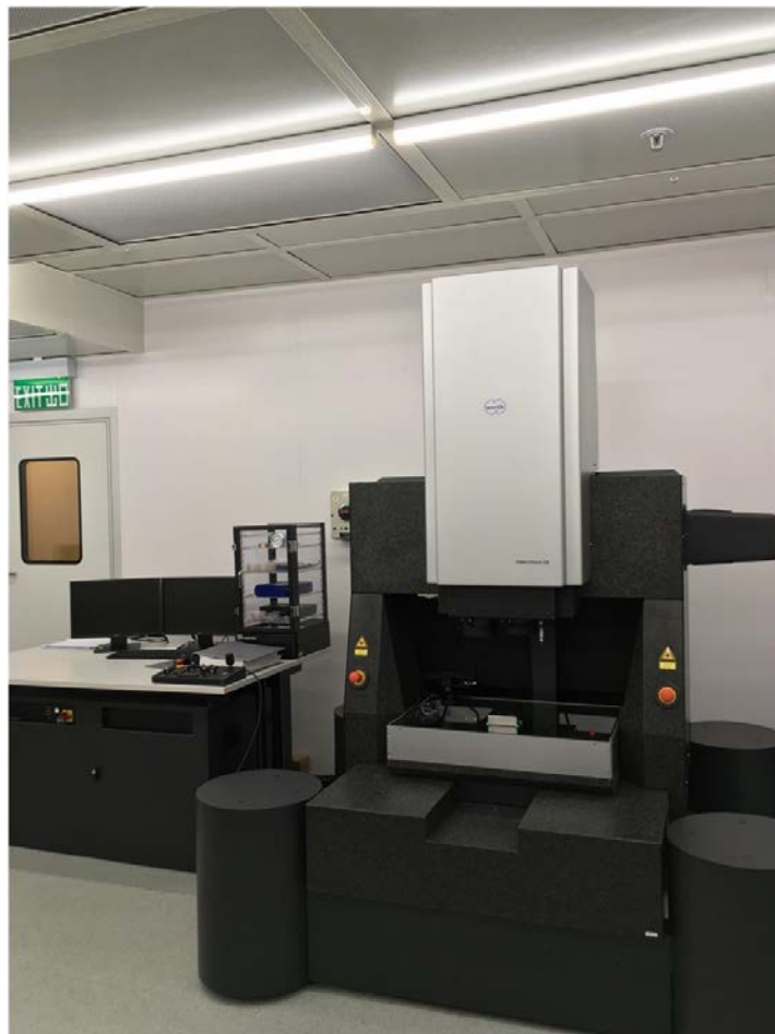
Figure 4.4 Werth VideoCheck UA multi-sensor CMM used for the experiments
