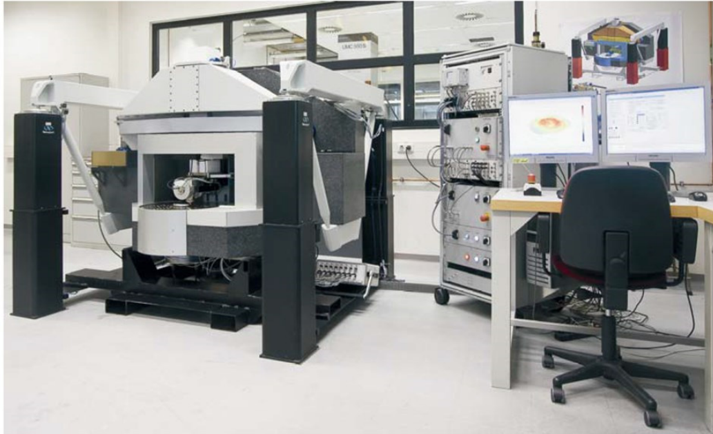
Figure 2.25 Non-contact freeform optics measurement machine prototype (Henselmans, 2009)
