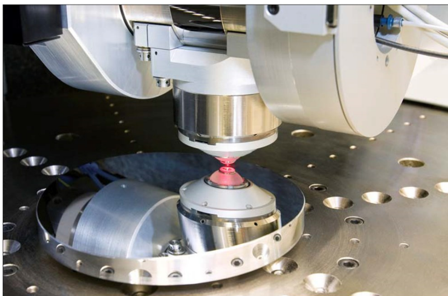
Figure 2.26 The optical sensor installed in the machine (Cacace, 2009)
