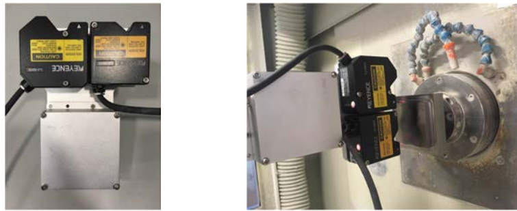
(a) Assembled sensor module (b) Installation in the machine tool
