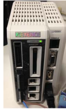
(b) LJ-G5001 controller for the laser sensor
