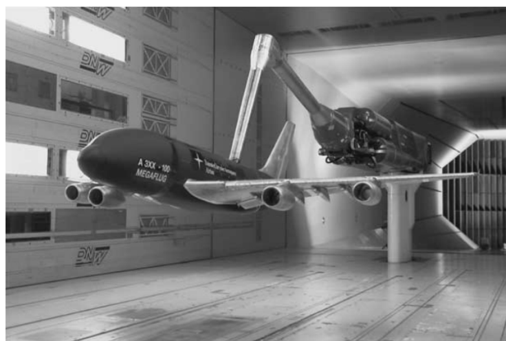
Figure 2.1 A complete model of airplane in the wind tunnel (Reckzeh, 2003)
