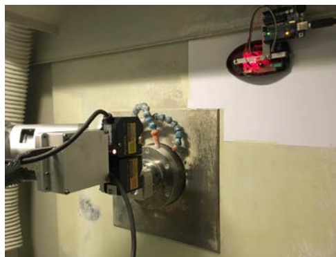
Figure 5.28 Optical motion sensor to detect the motion of the machine tool
