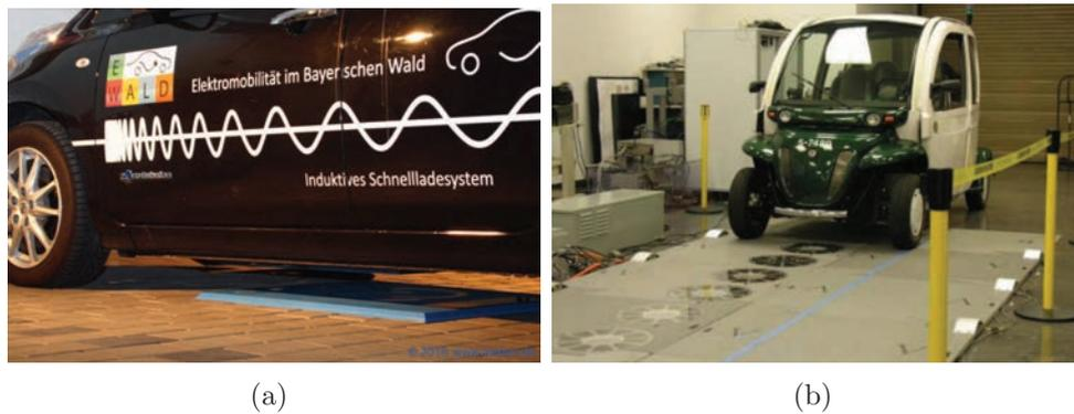
Figure 1.3: (a) A stationary EV charging system developed by INTIS [2], (b) A dynamic EV charging system developed by ORNL [3].
