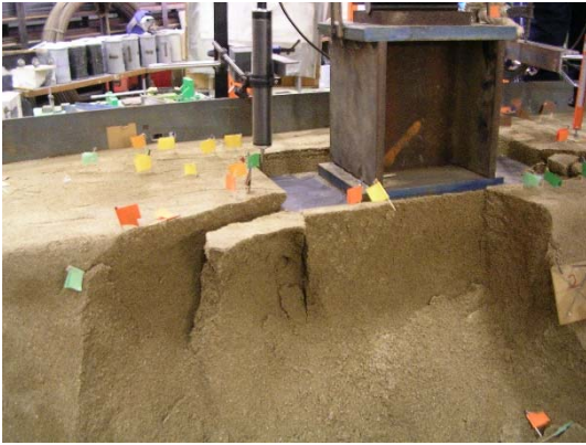
(a) Bearing failure beneath bearing plate
