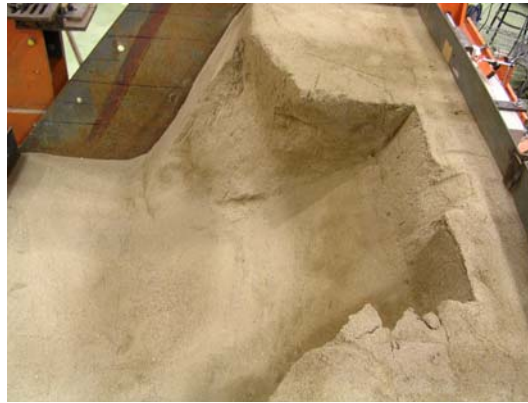
(b) Global three-dimensional failure beneath bearing plate
