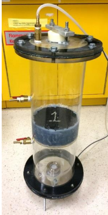
Figure 7.3 Part of the diffusion test system after being loaded with a specimen and sealed with Vaseline
