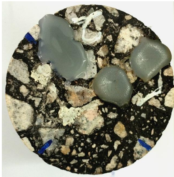
Figure 3.10 The holes of the control specimen after being filled with hot melt glue
