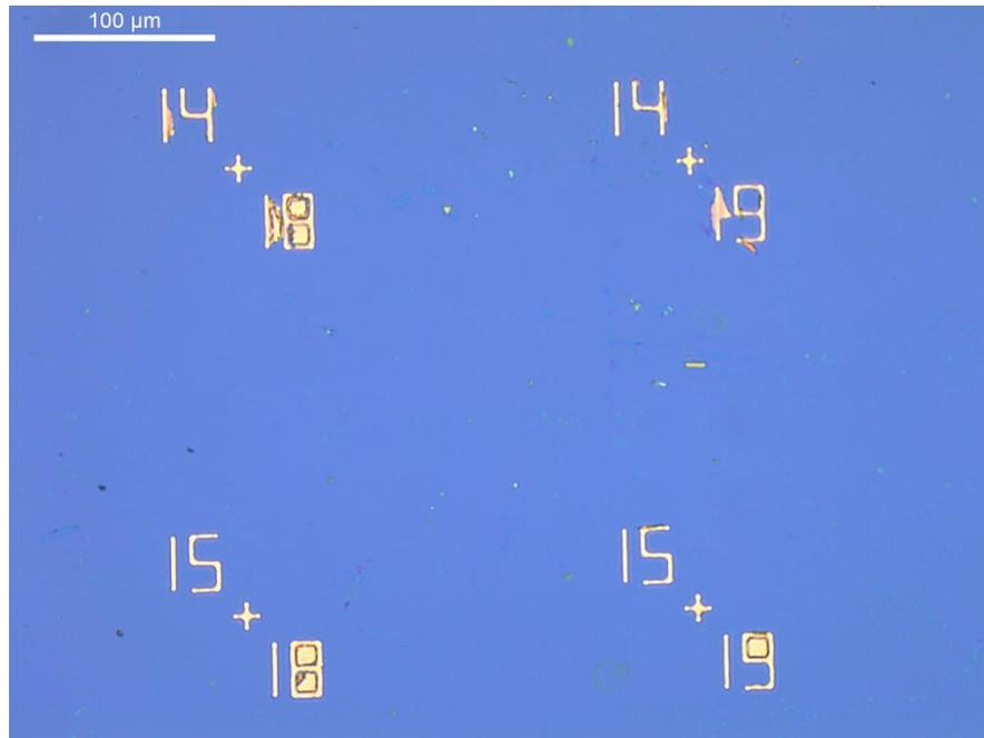
**Figure 4.1 Silicon Substrate Alignment Mark**
