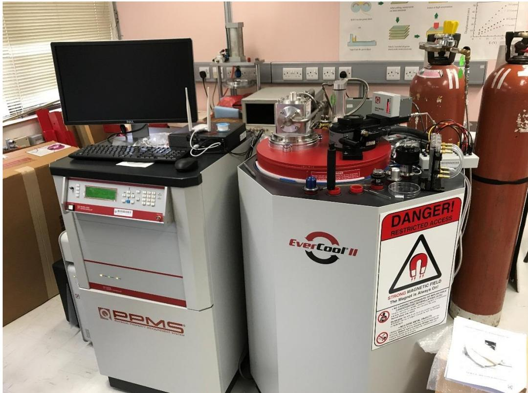
**Figure 2.14 Physical Property Measurement System**
