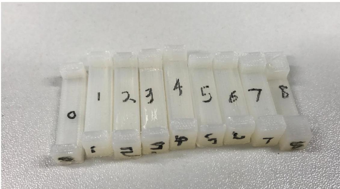
**Figure 3.4** Moulds built by 3D printer
