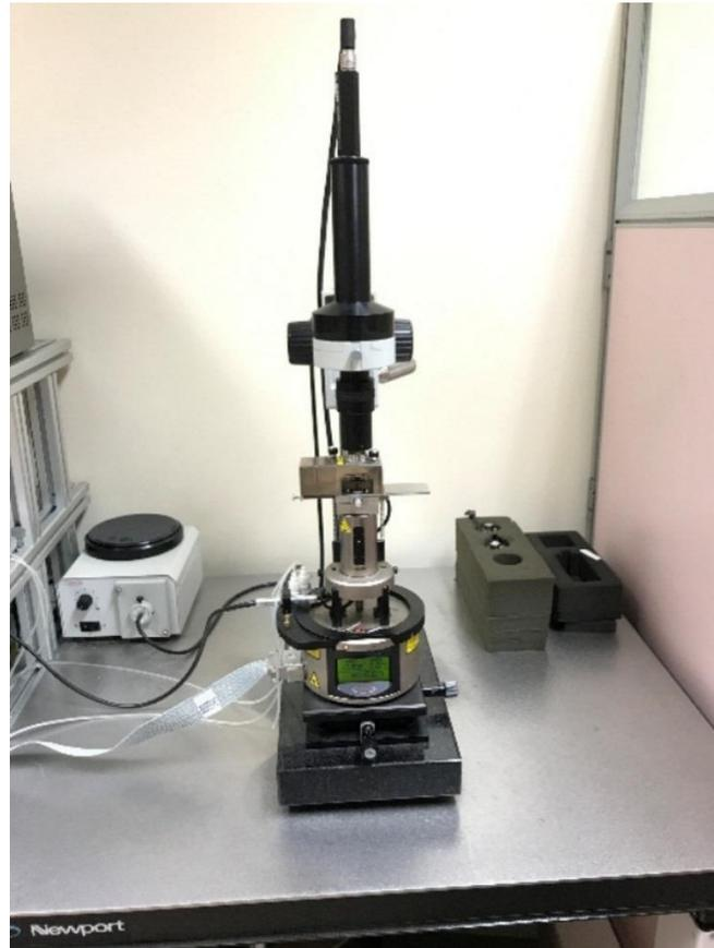
**Figure 2.8 Atomic force microscopy**
