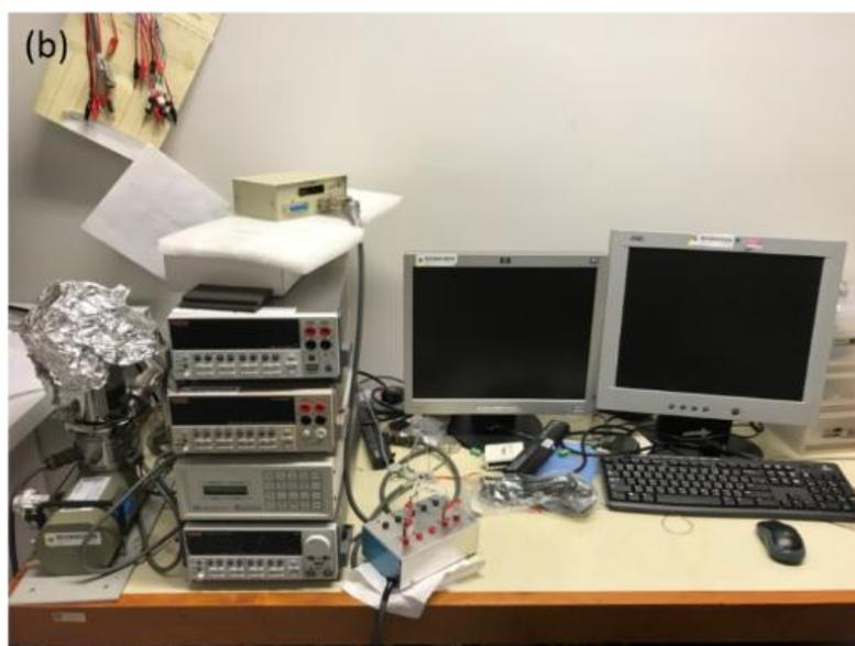
**Figure 2.12 (a) Two-point IV characterize curve measurement configuration (b) The experimental setup of Two-point IV characterize curve measurement**
