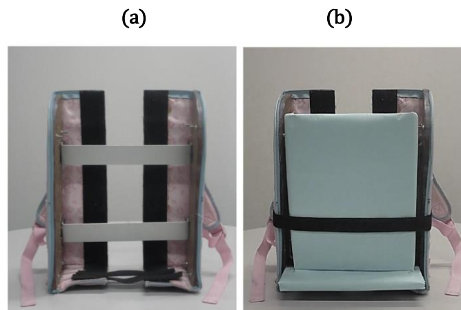
Figure 3.1 An internally reconstructed standard dual strap schoolbag. (a) The middle of its back was cut. (b) An internal frame was embedded and the level of center of gravity of the backpack was identified by a horizontal belt.
