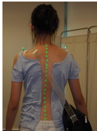
Figure 6.1 Digital anterior-posterior photo of participant 7 with the single-strap cross-chest bag placed on the contralateral side relative to the apex location and loaded at 5% of body weight. Circular markers were affixed to the spinous processes along the spine between C7 and L5.
