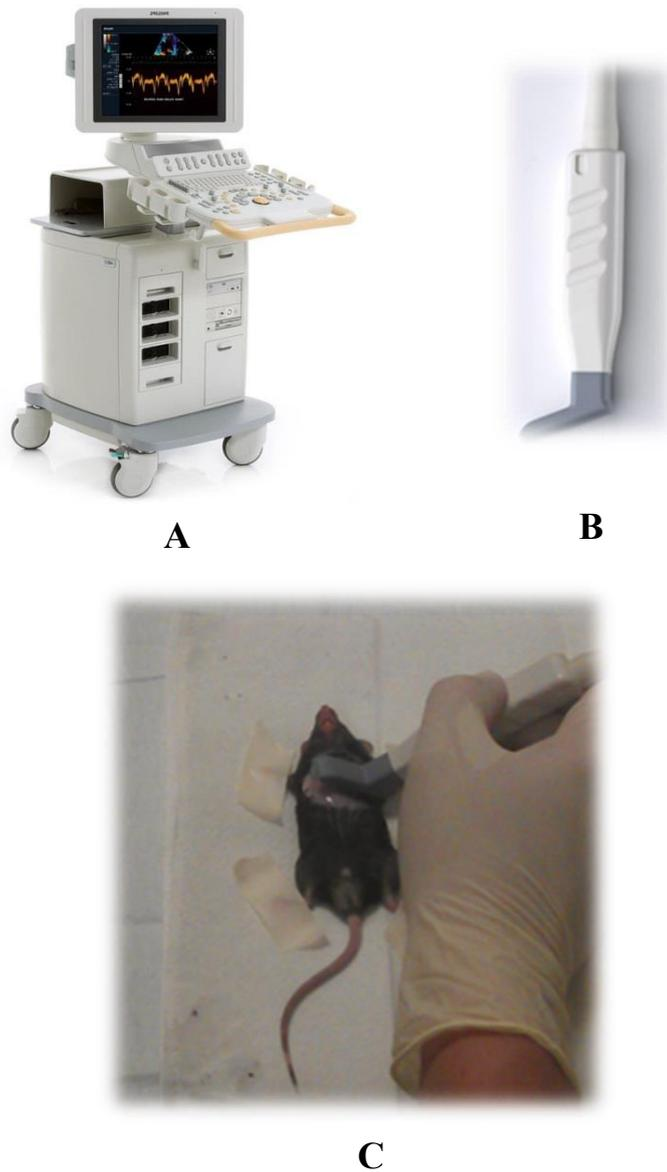
**Figure 2-2.** Equipment and technique used for mouse echocardiography.
