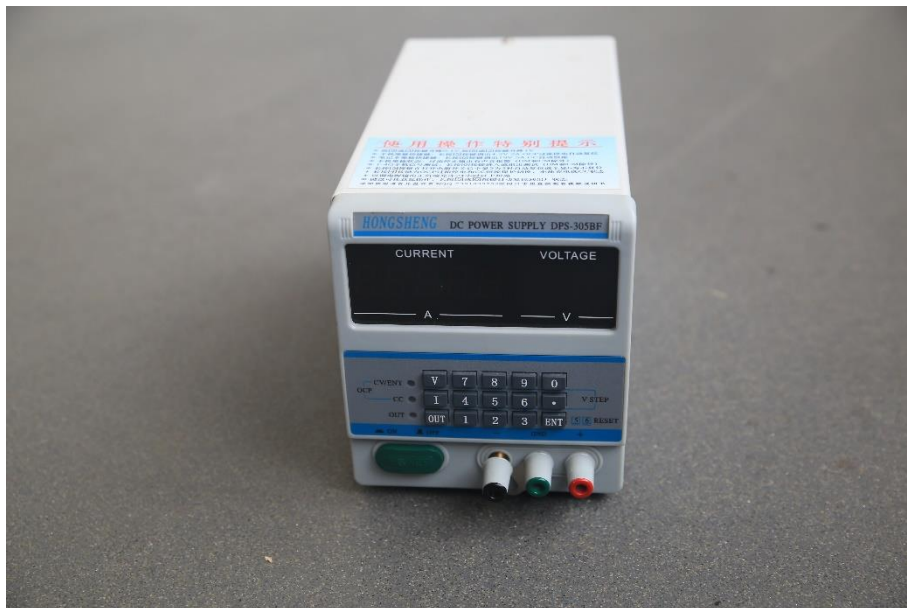
Figure 4.2 DC power supply for deposition experiment.
